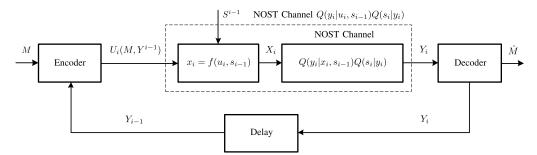
Fig. 7. An equivalent setting for the lower bound formulation with a new NOST channel Q(y|u, s')Q(s|y) where CSI is unavailable.
