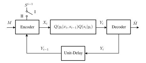
Fig. 1. NOST channels in the presence of feedback. Setting I (open switch) - no CSI is available. Setting II (closed switch) - CSI available at the encoder.
