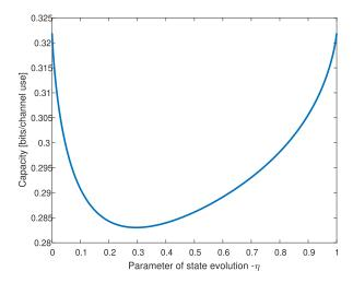
Fig. 5. The feedback capacity of the noisy-POST $(0.5, \eta)$  channel with or without CSI available at the encoder.
