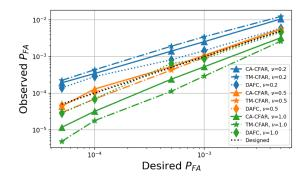
Fig. 10.  $P_{FA}$  verification for simulated clutter with "spikeness" levels  $\nu \in \{0.2, 0.5, 1\}$ . The desired  $P_{FA}$  denotes the false-alarm probability obtained using the validation dataset, and the observed  $P_{FA}$  denotes the false-alarm probability evaluated using the test dataset when the thresholds are according to the validation dataset.
