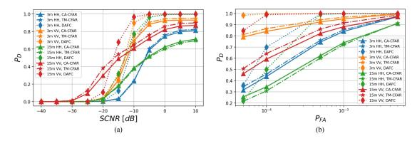
Fig. 11. Detection results in scenarios with targets and recorded radar clutter for 3 m and 15 m range resolutions, and VV and HH polarizations. Subplot (a) considers constant  $P_{\text{FA}} = 5 \cdot 10^{-4}$  and subplot (b) considers SCNR = 0 dB.
