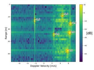
Fig. 1. Example of range–Doppler map containing simulated targets, clutter, and noise. The targets are circled in red, with the marked SCNRs. The nonhomogeneous clutter is present at the vicinity of the 4 m/s Doppler velocity in the majority of the range bins.
