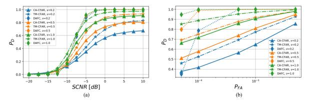
Fig. 8. Detection results with simulated clutter with embedded targets for various clutter "spikiness"  $\nu \in \{0.2, 0.5, 1.0\}$ . Subplot (a) considers constant  $P_{\text{FA}} = 5 \cdot 10^{-4}$  and subplot (b) considers SCNR = 0 dB.
