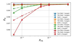
Fig. 5. ROC of evaluated detectors in clutter-free scenarios with  $\{1, 2, 4, 8\}$  targets and SCNR = 0 dB.
