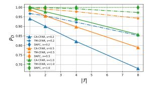
Fig. 9. Detection performance with simulated clutter as a function of the number of targets with SCNR = 0 dB and  $P_{\text{FA}} = 5 \cdot 10^{-4}$  for various clutter "spikeness"  $\nu \in \{0.2, 0.5, 1\}$ .
