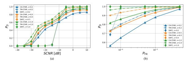
Fig. 7. Detection results with simulated clutter with targets for various clutter "spikiness"  $\nu \in \{0.2, 0.5, 1.0\}$ . Subplot (a) considers constant  $P_{\text{FA}} = 5 \cdot 10^{-4}$  and subplot (b) considers SCNR = 0 dB.
