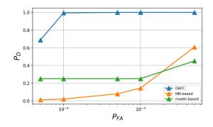
Fig. 13. ROC of various portions of the proposed algorithm with SCNR = 0 dB and simulated clutter with  $\nu = 0.5$ .
