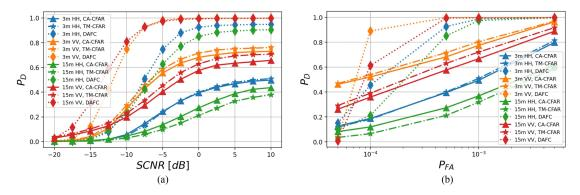
Fig. 12. Detection results in scenarios with embedded targets and recorded radar clutter for 3 m and 15 m range resolutions, and VV and HH polarizations. Subplot (a) considers constant  $P_{FA} = 5 \cdot 10^{-4}$  and subplot (b) considers SCNR = 0 dB.
