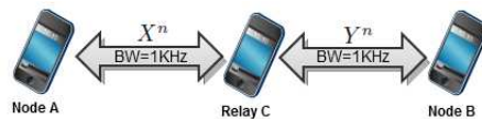
Fig. 1. This is a simple relay problem where bi-Directional communication between nodes A and B can be achieved only with the use of node C as a relay.
