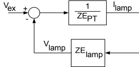
Figure 6. PT-CCFL ballast system represented as a feedback loop.
