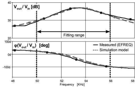
Figure 13. Comparison between measurement result (solid) and optimized model (dashed) input to output TR of experimental PT.
