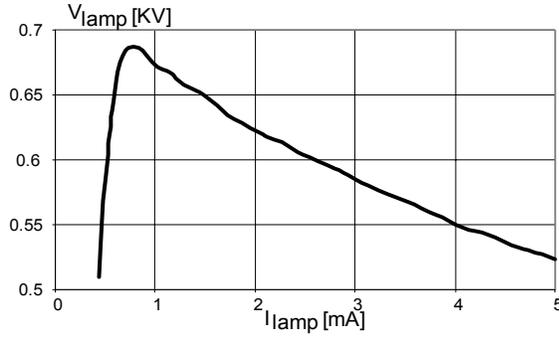
Figure 15. Measured static V-I curves of experimental CCFL (JKL BF3250-20B).
