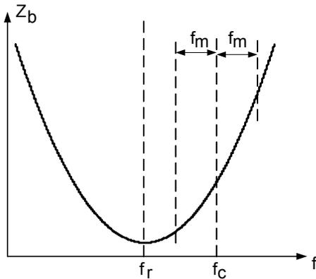
Figure 4. Impedance of a series resonant network, carrier frequency, and side bands.
