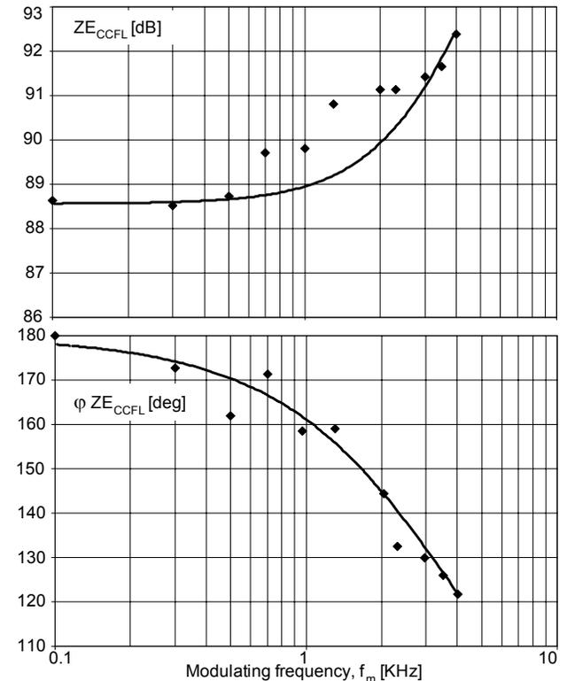
Figure 17. Measured (symbols) and simulated (solid lines) magnitude and phase EI of experimental CCFL (JKL BF3250-20B).
