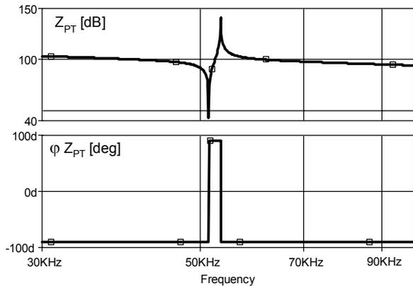
Figure 9. Output impedance of experimental PT.
