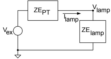
Figure 5. Simplified PT-CCFL ballast system.
