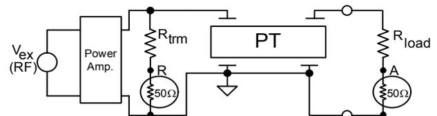
Figure 11. Experimental setup for input to output voltage transfer ratio measurements. The ratio A/R was measured by a network analyzer (HP4395A).
