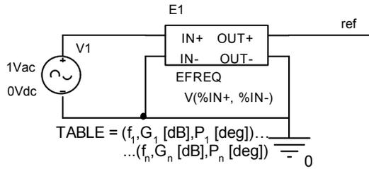
Figure 12. PSpice emulator of experimental TR of the PT. The table of the EFREQ dependent source lists the measured TR (magnitude and phase) over the measured frequency range.
