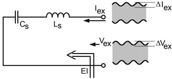
Figure 3. Illustrative explanation of the Envelope Impedance (EI) concept:  $EI(f) = \{\Delta V_{ex} / \Delta I_{ex}\}(f)$
