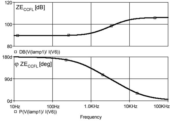
Figure 7. Envelope Impedance of experimental CCFL (JKL BF3250-20B).
