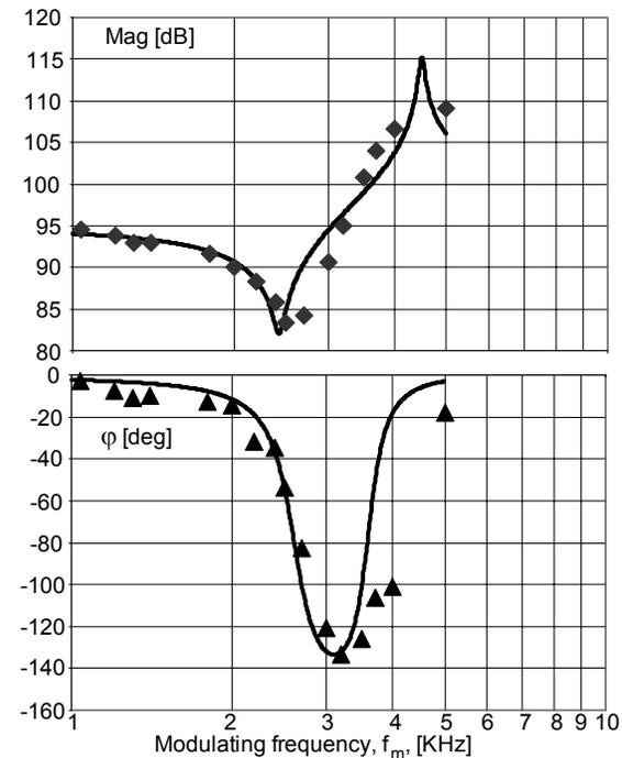
Figure 14. Measured (symbols) and simulated (solid lines) magnitude and phase EI of experimental PT (ELECERAM ELM-610). Carrier frequency: 49 KHz, resonant frequency: 51.5 KHz.
