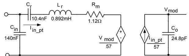
Figure 10. PT equivalent circuit and parameters.
