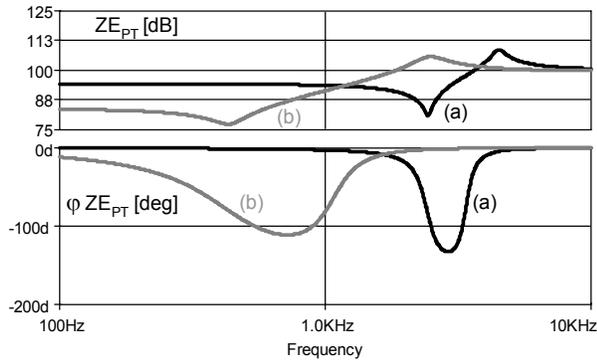
Figure 8. Envelope Impedance of experimental PT (ELECERAM ELM-610) for two carrier frequencies: (a) Operation far from output impedance resonance of the PT  $f_c=49$  KHz and (b) Operation near resonance  $f_c=51$  KHz. ( $f_r=51.5$  KHz)
