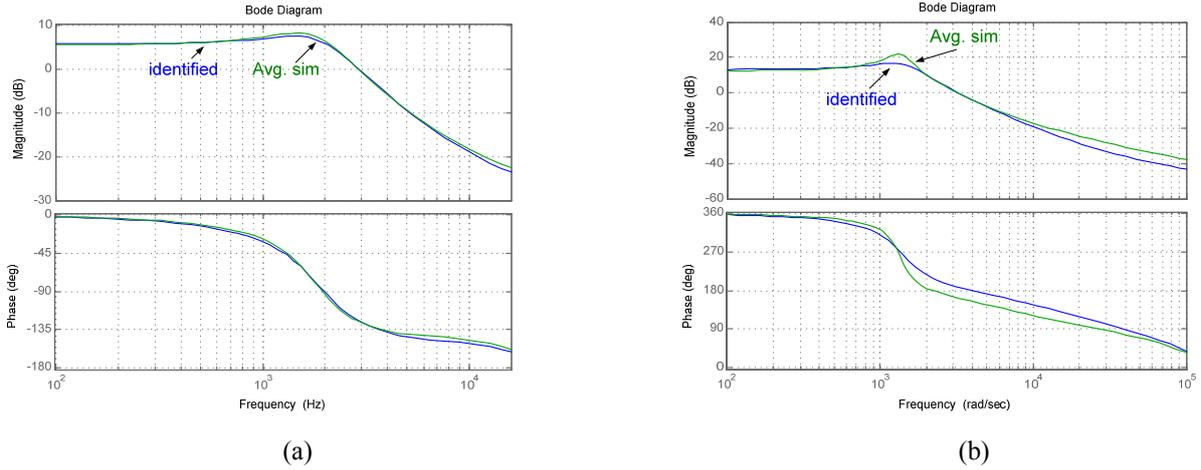
Figure. 7. Frequency response of the identified experimental converters compared to the frequency response of average simulation: (a) Buck converter (Eq. 4), (b) Boost converter (Eq. 5).
