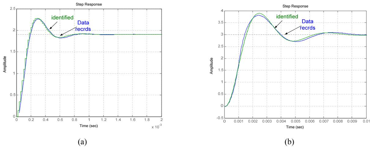
Figure. 5. Step response of the identified converters and original records obtained from the experimental system: (a) Buck converter (Eq. 4), (b) Boost converter (Eq. 5).
