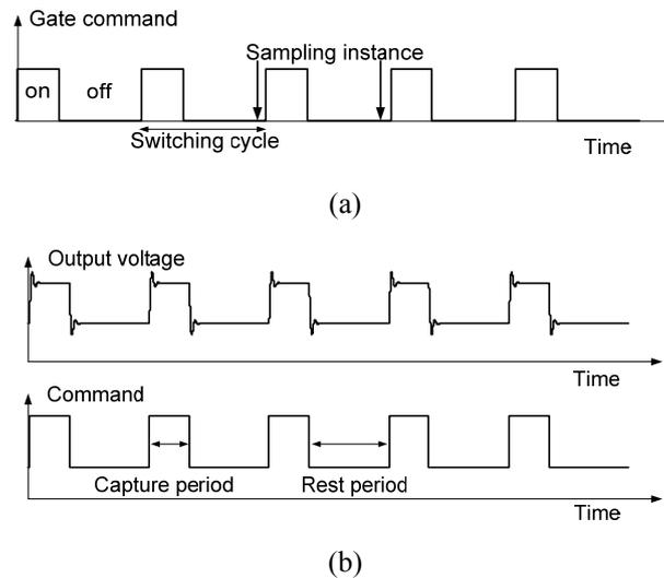
Figure. 3. Data acquisition details. (a) Sampling instance in relation to gate command. (b) Capture and rest periods.
