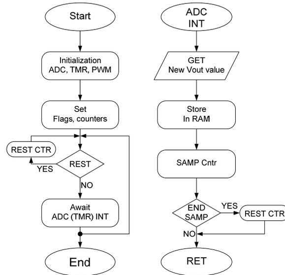
Figure 4. Sequenced data acquisition flowchart.
