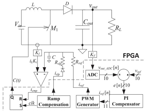
Fig. 1. Architecture of the FPGA-based CPM controller.
