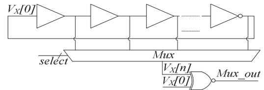
Fig.5. Construction of the FPGA-based HR DPWM
