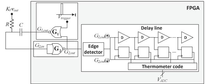
Fig.2. FPGA implementation of a delay-line ADC
