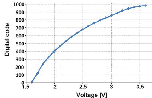
Fig.4. The static conversion characteristics of the experimental DL-ADC
