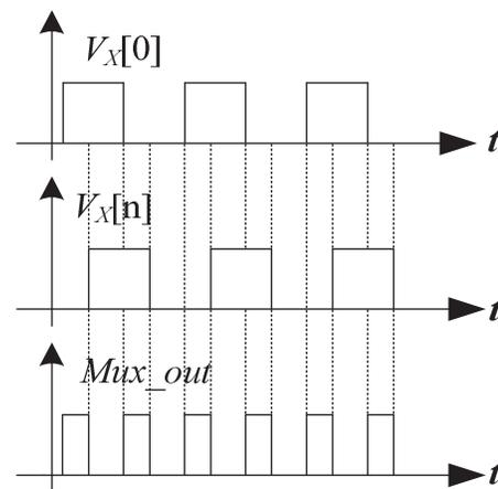
Fig.6. Operation of the FPGA-based HR DPWM
