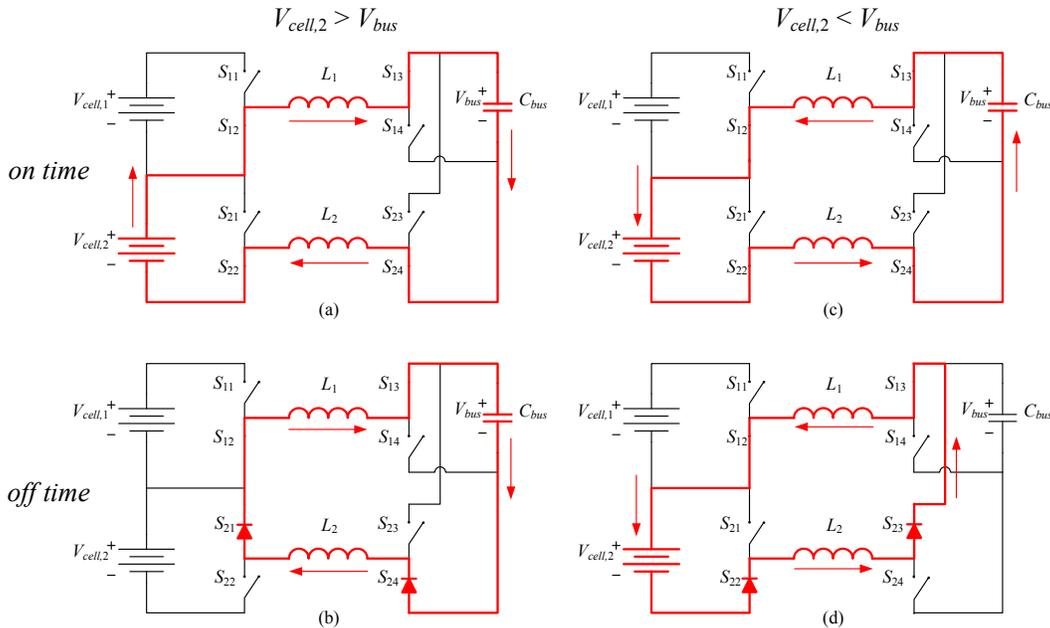
Fig. 6. Balancing operation of cell no. 2 for the case that  $V_{cell,2} > V_{bus}$ : (a) on time, (b) off time, and for the case that  $V_{cell,2} < V_{bus}$ : (c) on time, (d) off time.
