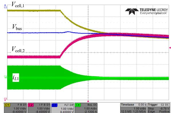
Fig. 12. Convergence of the cells' voltages for the case that  $V_{cell,1}$  and  $V_{cell,2}$  are preset to 12V and 8V, respectively. C1 –  $V_{cell,1}$  (1V/div), C2 –  $V_{cell,2}$  (1V/div), C3 –  $V_{bus}$  (1V/div), C4 – inductor current  $i_{L1}$  (1A/div). Time scale is 1s/div.
