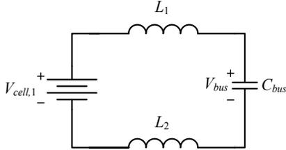
Fig. 3. The resultant circuit during on time when balancing  $V_{cell,1}$ .
