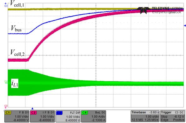
Fig. 11. Convergence of the cells' voltages when  $V_{cell,1}$  is connected to a 12V DC power supply;  $V_{cell,2}$  and  $V_{bus}$  converge toward  $V_{cell,1}$ . C1 –  $V_{cell,1}$  (1V/div), C2 –  $V_{cell,2}$  (1V/div), C3 –  $V_{bus}$  (1V/div), C4 – inductor current  $i_{L1}$  (1A/div). Time scale is 1s/div.
