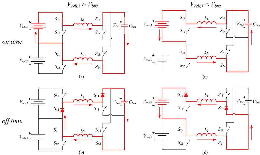
Fig. 4. Balancing operation of cell no. 1 for the case where  $V_{cell,1} > V_{bus}$ : (a) on time, (b) off time, and for the case where  $V_{cell,1} < V_{bus}$ : (c) on time, (d) off time. Arrows mark the current direction.
