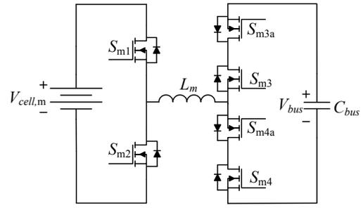
Fig. 8. Implementation of the switches for each balancing module with bidirectional switches using two MOSFETs.
