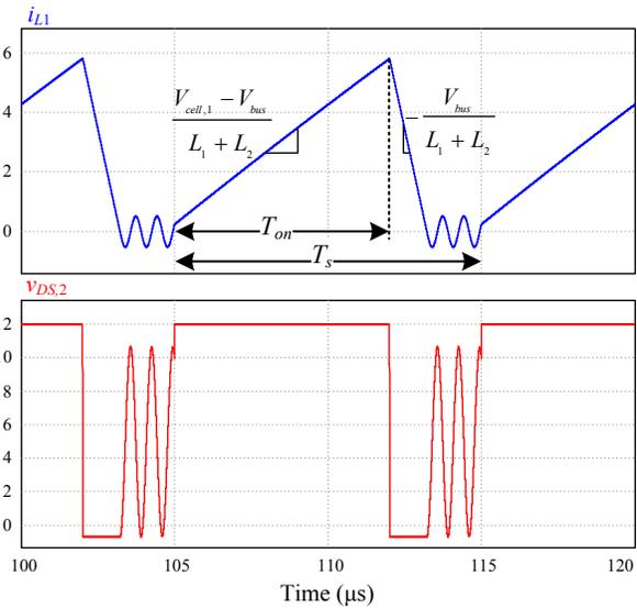
Fig. 5. Waveforms of the current in  $L_1$  and voltage across switch  $S_{12}$  when balancing cell no. 1 for the case that  $V_{cell,1} > V_{bus}$ .
