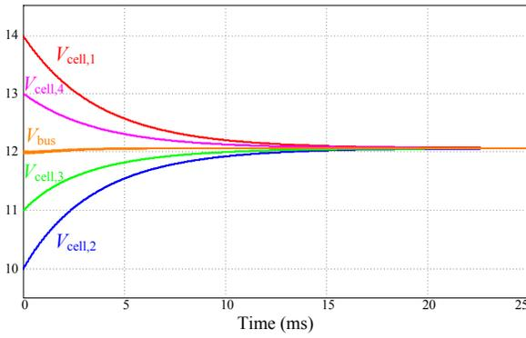
Fig. 7. Simulation results for 4 batteries cells emulated by large capacitors.
