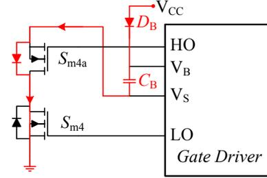
Fig. 9. Implementation of a bidirectional switch and an independent gate driver per transistor using a conventional bootstrapped driver. Bootstrap capacitor's current charging loop is marked in red.
