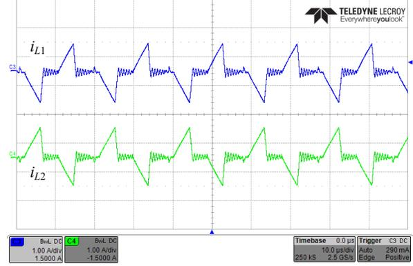
Fig. 10. Inductors currents for an unbalanced steady-state operation. C3 –  $i_{L1}$  (1A/div), C4 –  $i_{L2}$  (1A/div). Time scale is 10 $\mu$ s/div.
