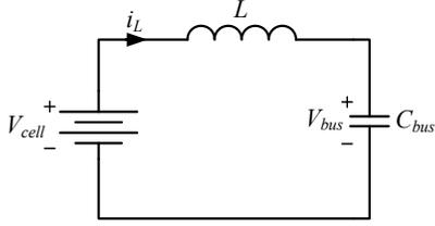
Fig. 2. Voltage equalizing mechanism of a battery cell and the bus capacitor.
