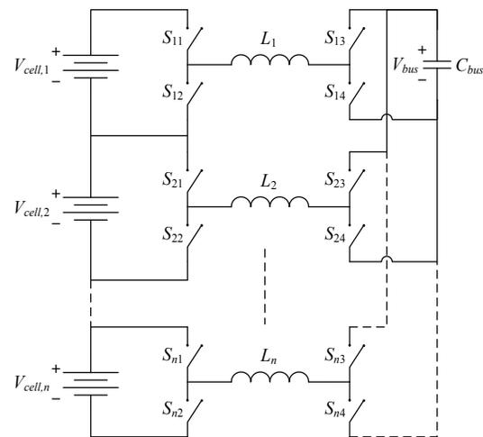
Fig. 1. Batteries balancing system for  $n$  serially connected batteries.
