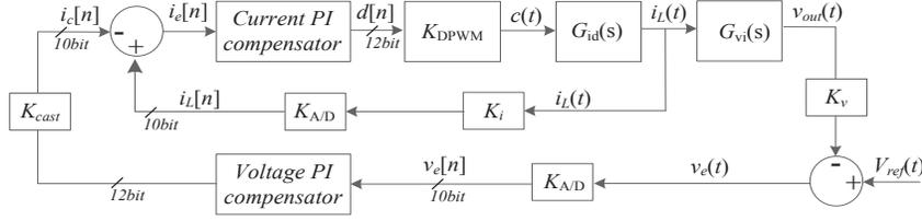
Fig. 2. System block diagram including the buck converter and ACM controller corresponding gains.
