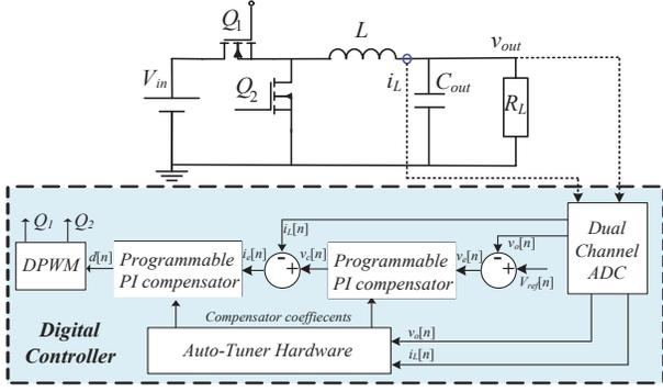
Fig. 1. Simplified diagram of a synchronous buck converter with the digital auto-tuning ACM controller.
