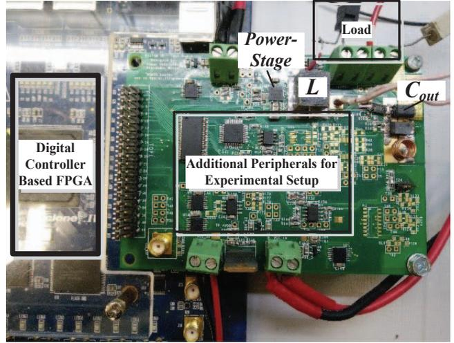
Fig. 5. Experimental prototype for evaluation of the auto-tuning ACM controller. The controller and tuner are realized on FPGA, PCB comprises a synchronous buck converter and additional periphery for signal integrity.
