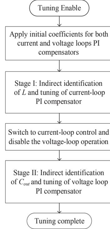
Fig. 3. Flowchart of the controller's tuning procedure.
