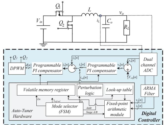
Fig. 4. Full block diagram of the digital auto-tuning ACM controller.
