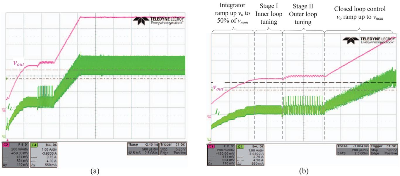
Fig. 6. Experimental results of the soft-start period with auto-tuning: (a) soft-start and regulation, (b) zoom in on the tuning procedure ( $V_{out}$  200mV/div,  $i_L$  1A/div, time scale is 200 $\mu$ s/div).
