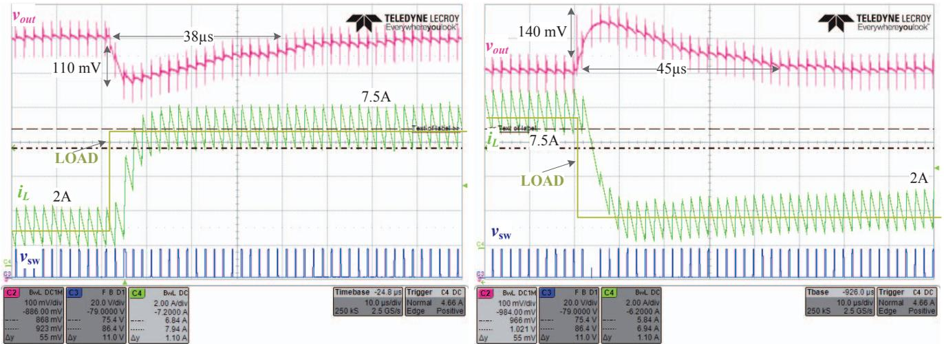
Fig. 7. Experimental load steps of 5.5A with 1 $\mu$ H inductor and 100 $\mu$ F ceramic output capacitor ( $v_{out}$  100mV/div,  $i_L$  2A/div,  $V_{sw}$  20V/div, time scale is 10 $\mu$ s/div).
