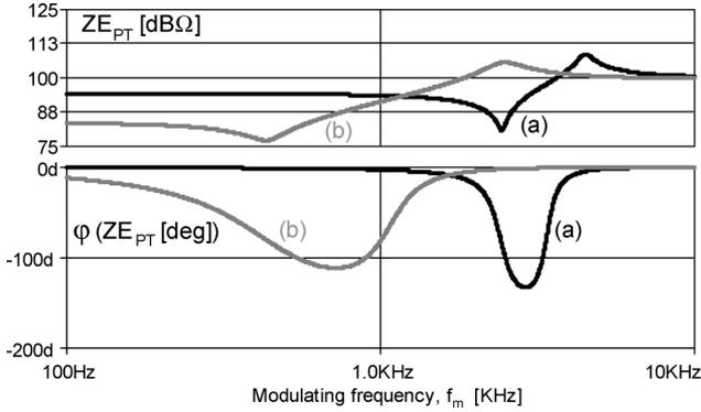
Fig. 9. Envelope Impedance of experimental PT (ELECERAM ELM-610) for two carrier frequencies: (a) operation far from output impedance resonance of the PT  $f_c = 49$  KHz and (b) operation near resonance  $f_c = 51$  KHz ( $f_r = 51.5$  KHz).
