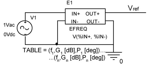
Fig. 13. PSpice emulator of experimental TR of the PT. The table of the EFREQ dependent source lists the measured TR (magnitude and phase) over the measured frequency range.
