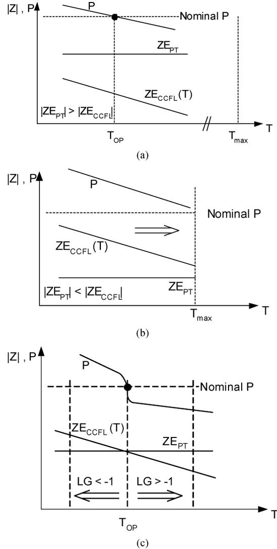
Fig. 20. Possible modes of operation of PT-CCFL system: (a)  $f_c$  far from  $f_r$ , stable mode and (b)  $f_c = f_r$  unstable mode and (c)  $f_c$  near  $f_r$ , oscillations mode.
