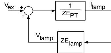
Fig. 7. PT-CCFL ballast system represented as a feedback loop.
