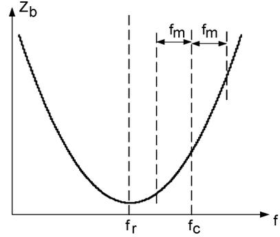
Fig. 5. Impedance of a series resonant network, a carrier frequency, and side bands.
