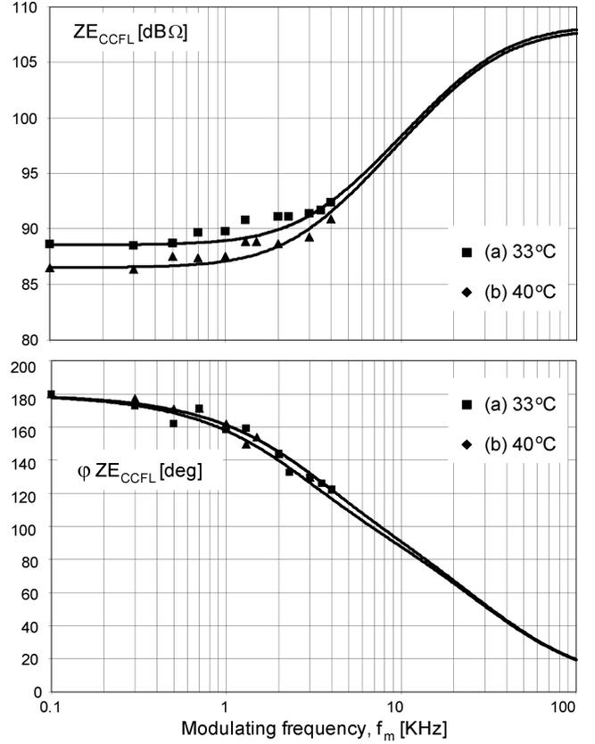
Fig. 18. Measured (symbols) and simulated (solid lines) magnitude and phase EI of experimental CCFL (JKL BF3250-20B) in two thermal bias points: (a)  $33^\circ\text{C}$  and (b)  $40^\circ\text{C}$ .
