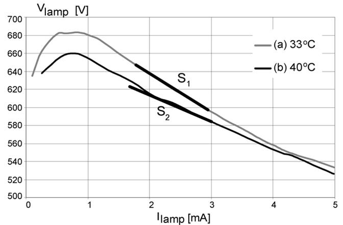
Fig. 16. Measured static  $V-I$  curves of experimental CCFL (JKL BF3250-20B) operating in two thermal bias points: (a) 33 °C. (b) 40 °C.
