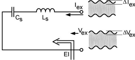
Fig. 4. Illustrative explanation of the envelope impedance (EI) concept:  $EI(f) = \{\Delta V_{ex} / \Delta I_{ex}\}(f)$ .
