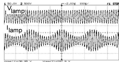
Fig. 2. Measured CCFL voltage (0.5 kV/div) and current (3.3 mA/div) when driven by a PT based HF electronic ballast. Horizontal scale 0.1 ms/div.
