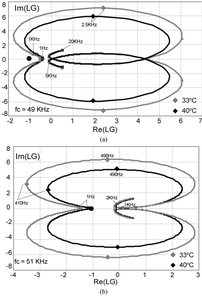
Fig. 19. Nyquist plots of experimental PT-CCFL system under different operating conditions (carrier and thermal wise): (a) carrier frequency is far from resonance, stable operation in both thermal operating points and (b) carrier frequency near resonance, 40 °C: stable operation, 33 °C: unstable operation.
