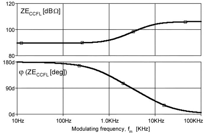
Fig. 11. Envelope Impedance of experimental CCFL (JKL BF3250-20B).
