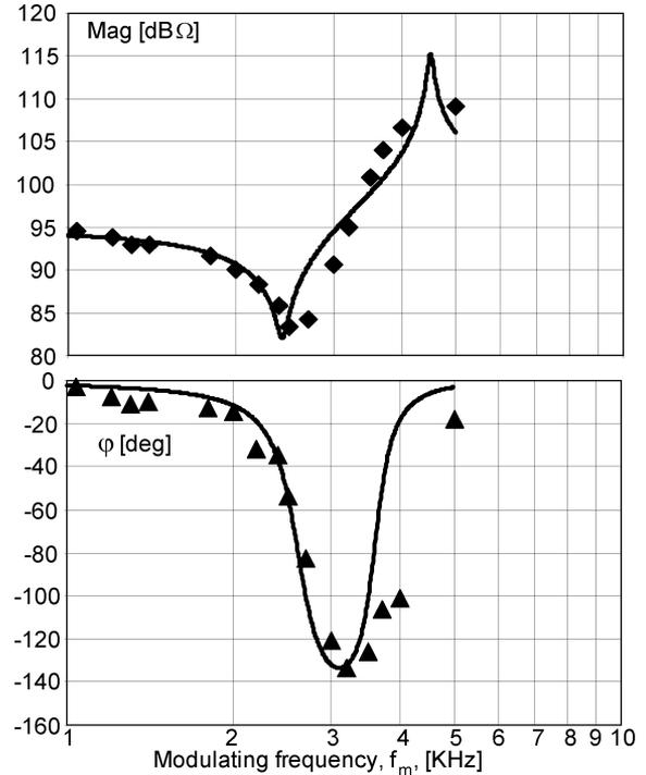
Fig. 15. Measured (symbols) and simulated (solid lines) magnitude and phase EI of experimental PT (ELECERAM ELM-610). Carrier frequency: 49 KHz, resonant frequency: 51.5 KHz.
