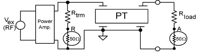
Fig. 12. Experimental setup for input to output voltage transfer ratio measurements. The ratio A/R was measured by a network analyzer (HP4395A). The  $50 \Omega$  resistors represent the input resistance of the network analyzer.
