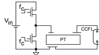
Fig. 1. PT-CCFL ballast system driven by half-bridge power stage.
