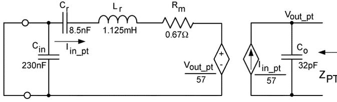
Fig. 8. PT equivalent circuit and parameters, connected in the output impedance measurement setup.
