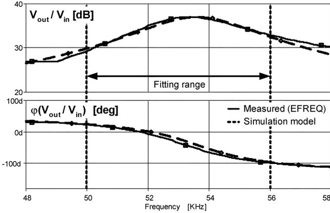
Fig. 14. Comparison between measurement result (solid) and optimized model (dashed) input to output TR of experimental PT.
