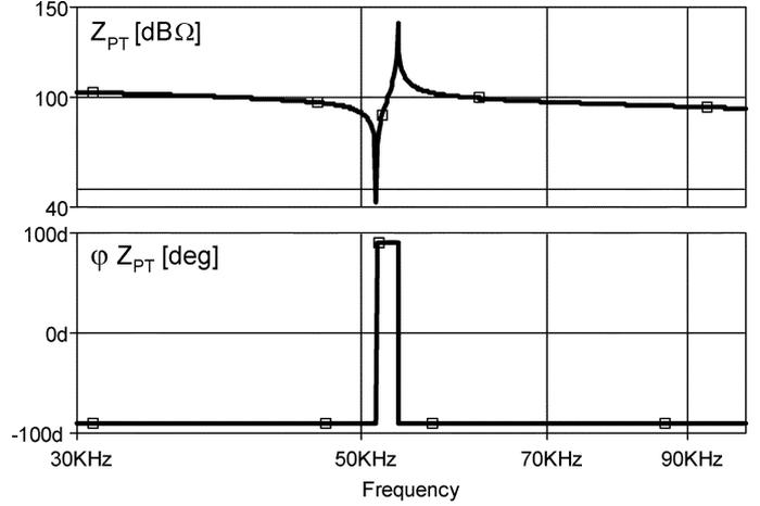
Fig. 10. Output impedance of experimental PT.
