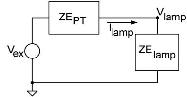
Fig. 6. Simplified PT-CCFL ballast system.
