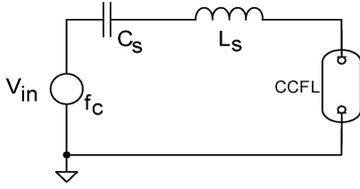
Fig. 3. CCFL driven by a HF resonant ballast.
