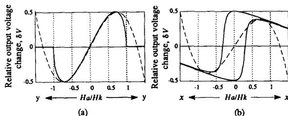
Fig. 2. Theoretical transfer characteristics of differential barber-pole MR sensor (broken lines are approximation curves). (a) hard-axis characteristic. (b) easy-axis characteristic (dc biases  $H_{bx}$  and  $H_{by}$  of appropriate sizes are applied along the easy axis and along the hard axis of the sensor respectively).
