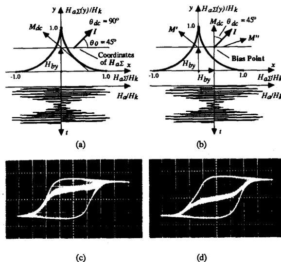
Fig. 3. (a), (b) astroid models of the multifield excited MR sensor. (c), (d) experimental outputs of the MR sensor vs excitation field.  $X = 100$  (A/m)/div;  $Y = 50$  mV/div. (a), (c) dc bias field  $H_{by}$  is applied along the sensor hard axis only; (b), (d) purely odd characteristic is obtained when appropriate dc biases  $H_{bx}$  and  $H_{by}$  are applied along both sensor axes.
