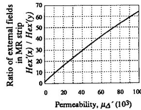
Fig. 4. Ratio of the magnetic field along the easy axis to that along the hard axis vs apparent incremental permeability.
