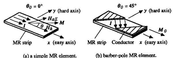
Fig. 1. Geometry of MR sensors.
