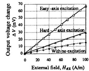
Fig. 5. Experimental output characteristics of the MR sensor.
