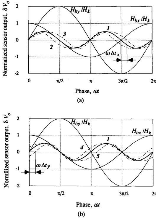
Fig. 3. The theoretical outputs of the magnetoresistive sensor employing rotating excitation. The outputs are obtained for different values of dc external field. (a)  $H_{uy} = 0$ ; 1 -  $H_u = 0$ ; 2 -  $H_{ux} < 0$ ; 3 -  $H_{ux} > 0$ . (b)  $H_{ux} = 0$ ; 4 -  $H_u = 0$ ; 5 -  $H_{uy} < 0$ ; 5 -  $H_{uy} > 0$ .
