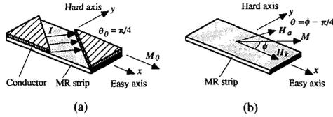
Fig. 1. Barber-pole magnetoresistor. (a) Geometry of a barber-pole magnetoresistive element. ( $\theta_0$ : the angle between the quiescent direction of the magnetization and the current through the magnetoresistive stripe;  $M_0$ : the quiescent magnetization). (b) Magnetization in a magnetoresistive stripe.
