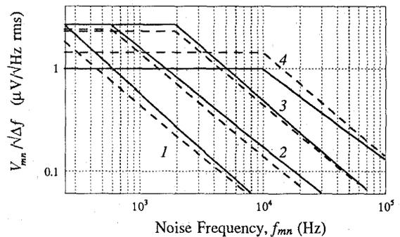
Fig. 4. Simplified representation of the spectra in Fig. 3. Dashed lines show the theoretically obtained spectra of the magnetic-noise voltage.
