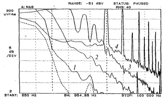
Fig. 3. Experimentally obtained spectra of the magnetic noise produced by KMZ10 type magnetoresistor. 1 -  $f_{ex} = 10$  Hz, 2 -  $f_{ex} = 100$  Hz, 3 -  $f_{ex} = 1$  kHz, 4 -  $f_{ex} = 10$  kHz. Dashed line shows spectrum of the total noise induced by the measuring system and the environment.
