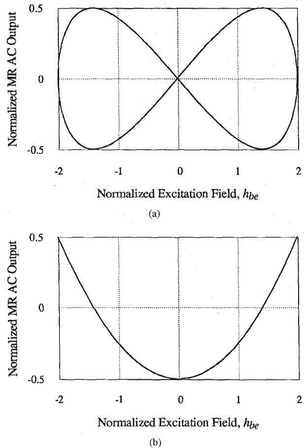
Fig. 4. The theoretically obtained outputs (normalized MR ac output versus normalized easy-axis excitation field) of magnetoresistors employing rotating excitation method described in [1]. (a) Output signal of barber-pole magnetoresistor. (b) Output signal of unbiased magnetoresistor.
