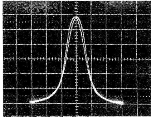
Fig. 8. Output characteristic (MR ac output versus hard-axis magnetic field) of the unbiased magnetoresistor.  $X = 1$  (kA/m)/div;  $Y = 5$  mV/div.
