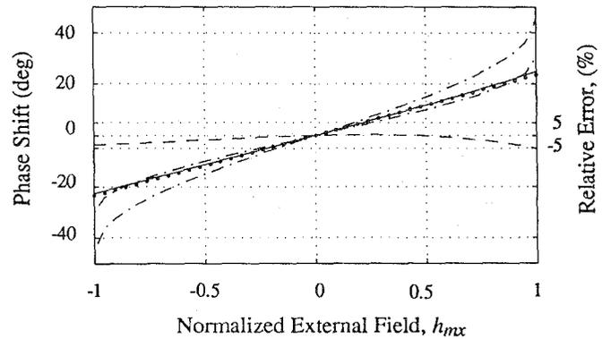
Fig. 7. Theoretical response characteristic (dotted line) of unbiased magnetoresistor employing the proposed rotating excitation method. For comparison we also show the theoretically obtained easy-axis and hard-axis response characteristics (dashed-dotted lines) of barber-pole magnetoresistor employing the rotating excitation method described in [1]. The solid line is a linear approximation of the response characteristic. The broken line represents the relative error of the approximation.
