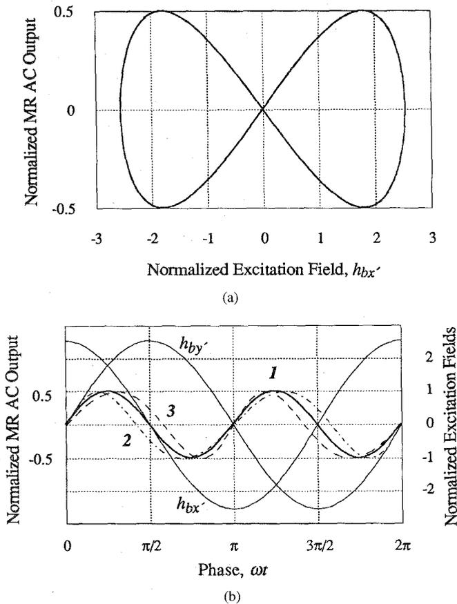
Fig. 6. The theoretically obtained outputs of an unbiased magnetoresistor employing the proposed rotating excitation method. (a) Magnetoresistive output versus the easy-axis excitation field. (b) Magnetoresistive outputs versus time. The outputs are obtained for different values of dc external field: 1— $H_{mx} = 0$ ; 2— $H_{mx} < 0$ ; 3— $H_{mx} > 0$ ; 1-3— $H_{my} = 0$ .
