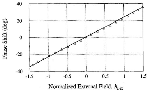
Fig. 11. The experimental and theoretical (solid line) response characteristics of the unbiased magnetoresistor that employs the proposed rotating excitation.
