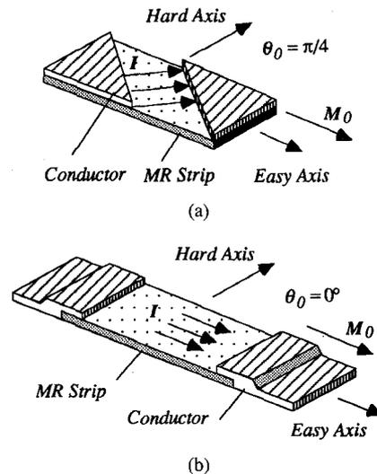
Fig. 1. Magnetoresistors. (a) Geometry of a barber-pole magnetoresistive element. (b) Unbiased magnetoresistor. [ $\theta_0$ —the angle between the quiescent magnetization ( $M_0$ ) direction and the current through the magnetoresistive strip.]
