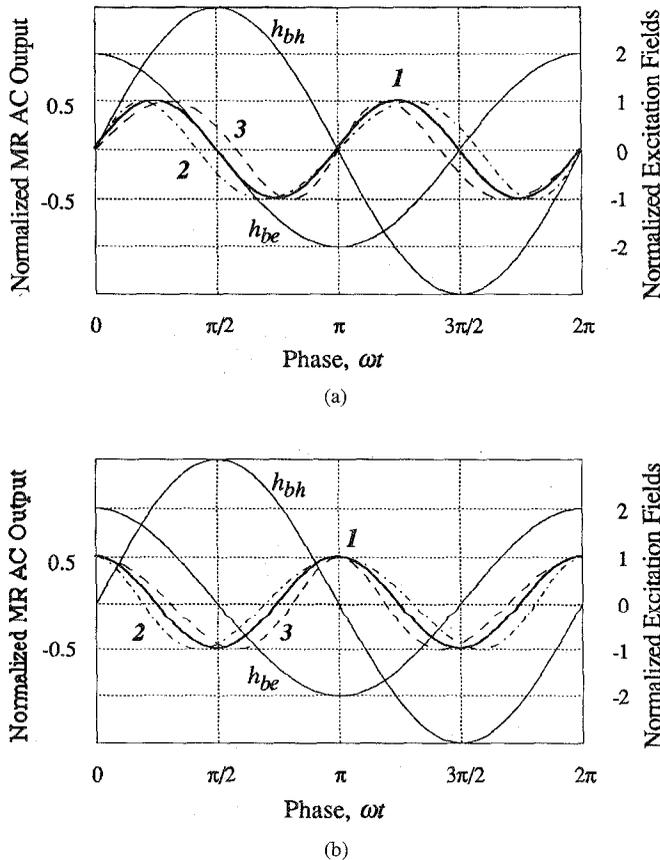
Fig. 3. The theoretically obtained outputs (normalized MR ac output versus time) of magnetoresistors employing rotating excitation method described in [1]. (a) Output signals of barber-pole magnetoresistor. (b) Output signals of unbiased magnetoresistor. The outputs are obtained for different values of dc external field: 1— $H_{mx} = 0$ ; 2— $H_{mx} < 0$ ; 3— $H_{mx} > 0$ ; 1-3— $H_{my} = 0$ .
