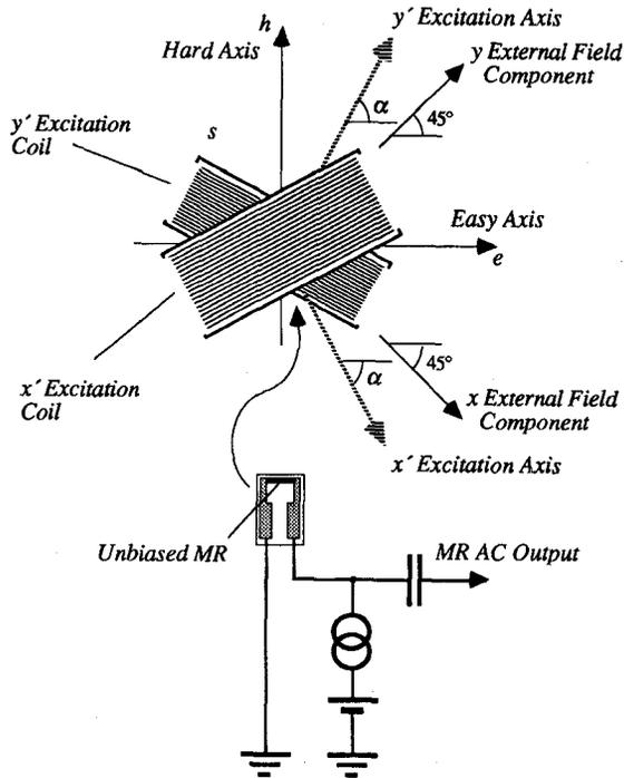
Fig. 5. Schematic diagram of the experimental setup devised for excitation of an unbiased magnetoresistor by rotating field according to the presently proposed method.
