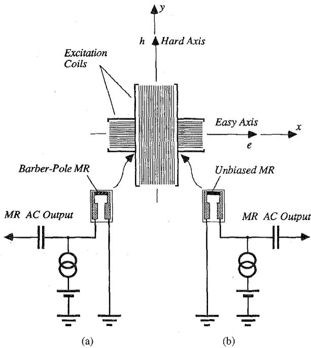
Fig. 2. Schematic diagram of the experimental setup for exciting magnetoresistors by rotating field as was proposed in [1]. (a) Excitation of barber-pole magnetoresistor. (b) Excitation of unbiased magnetoresistor.
