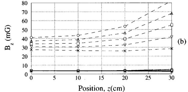
FIG. 7. Effectiveness of the proposed method. (a) Residual magnetic field measured along the shield axis taking radial position  $x$  as a parameter (compensation is on:  $I_1=0.8$  A;  $I_2=1.2$  A). (b) A comparison between the data shown in Fig. 2 (the dashed curves) and (a).
