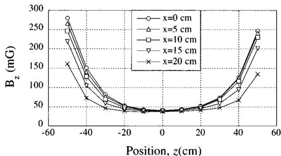
FIG. 2. Residual magnetic field measured along the shield axis taking radial position  $x$  as a parameter (compensation is off:  $I_1=0$ ;  $I_2=0$ ).
