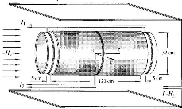
FIG. 1. Schematic layout of the shielding system.
