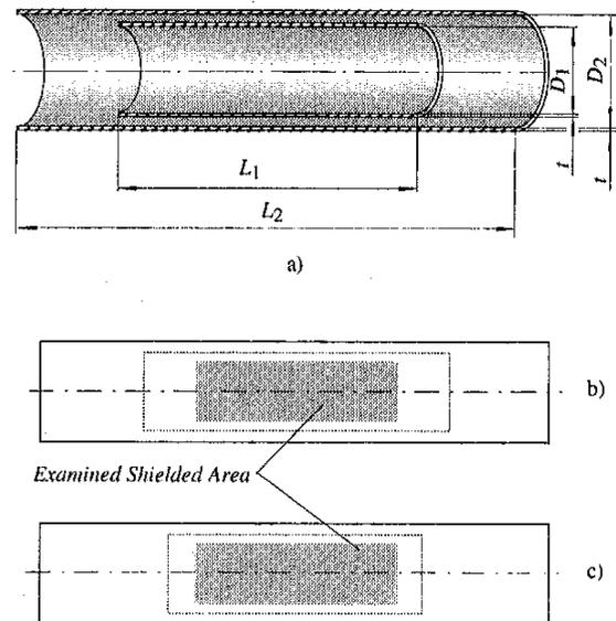
Fig. 3. Double-shell open-ended cylindrical shield. Shields' dimensions:  $L_2/D_2=5$ ,  $D_1/D_2=0.8$ ,  $t_1=t_2=0.01 \cdot D_2$ ,  $\mu_1=\mu_2=10,000$ , b)  $L_1/L_2=0.6$ , c)  $L_1/L_2=0.5$ . Examined shielded area:  $L_a=2 \cdot D_2$ ,  $D_a=0.6 \cdot D_2$ .
