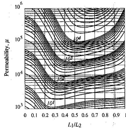
Fig. 5. Axial shielding factor of double-shell open-ended cylindrical shield as a function of the inner shell to outer shell lengths ratio,  $L_1/L_2$ , and permeability,  $L_2/D_2=5$ ,  $D_1/D_2=0.8$ ,  $t_1=t_2=0.01 \cdot D_2$ . [4].
