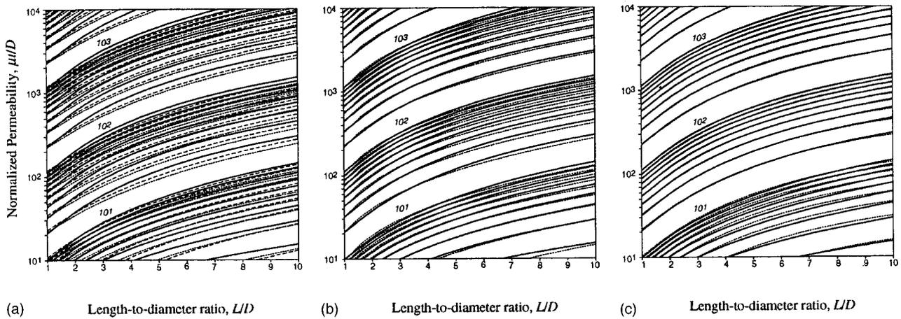
FIG. 2. The axial shielding factors for single-shell closed cylindrical shields: numerical results (solid lines) and analytical results predicted in (a) by Eq. (2) (dotted lines) and the theory in Ref. 1 (dashed lines), in (b) by Eq. (4) where  $f=1$  (dotted lines), and in (c) by Eq. (4) where  $f=1+(L/D)/100$  (dotted lines).
