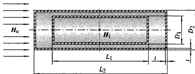
FIG. 1. Double-shell closed cylindrical magnetic shield.
