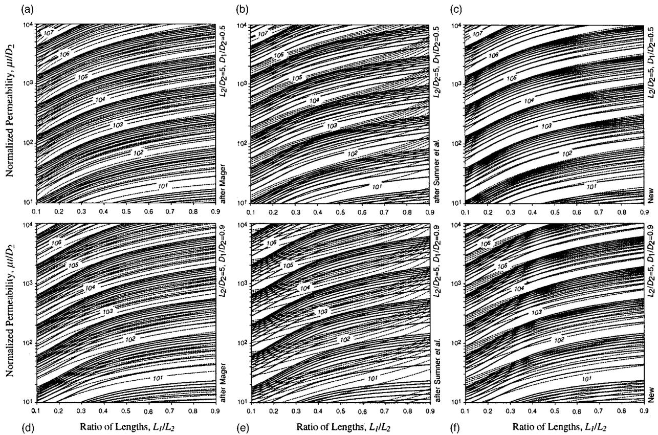
FIG. 4. The axial shielding factors for double-shell closed cylindrical shields: numerical results (solid lines) and analytical results (dotted lines) predicted in (a), (d) by Eq. (1), in (b), (e) by Eq. (3), and in (c), (f) by Eqs. (4) and (5). Equation (5) well approximates the numerical results for all the numerical models we tested (a representative example is shown).
