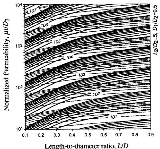
FIG. 3. The axial shielding factors for double-shell closed cylindrical shields: numerical results (solid lines) and analytical results (dotted lines) predicted by Eq. (1). An enormous difference is observed for all the numerical models (a representative example is shown).
