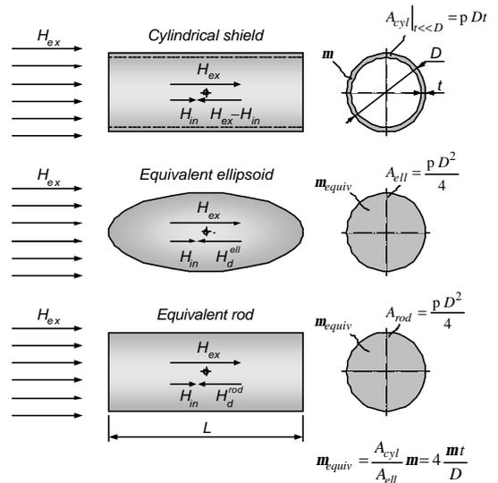
Fig. 1. Magnetic field reduction,  $H_{ex} - H_{in}$ , at the center of a cylindrical shield, the equivalent ellipsoid and rod (the effect of the shield openings is neglected).
