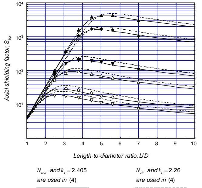
Fig. 6. Axial shielding factor of open cylindrical shields as function of their aspect ratio,  $L/D$ : a comparison between the experimental and theoretical results. This figure shows that the experimental data is better approximated by (4) where the demagnetizing factor for rod rather than for ellipsoid is used.
