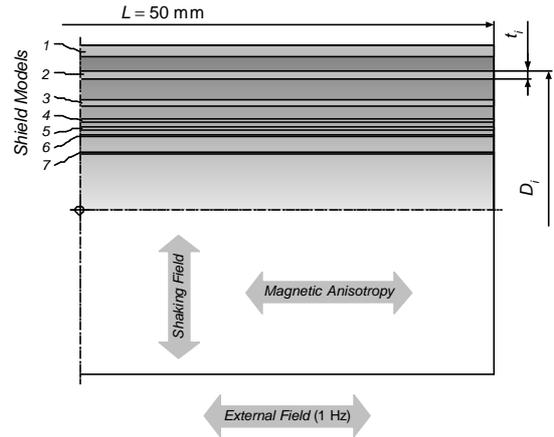
Fig. 4. Experimental shield models. (The models are shown as a coaxial assembly, although each cylinder was examined separately as a single-shell shield.) This figure illustrates that the thickness of each cylinder is directly proportional to its diameter, thus, keeping a constant  $t/D=1/45.5$  ratio for all the models.
