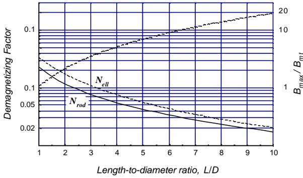
Fig. 2. Demagnetizing factors for ellipsoid and rod as a function of their aspect ratio,  $L/D$ . Ratio of maximum flux densities in axial and transverse magnetic shields,  $B_{max}/B_{mt}$ , as a function of the aspect ratio,  $L/D$ .
