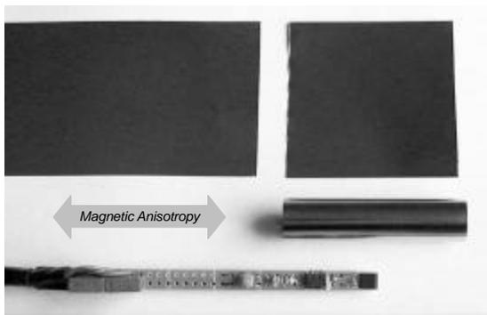
Fig. 3. A miniature shield model made of 50x50 mm pieces cut from 22  $\mu\text{m}$ -thick amorphous Metglas 2705M ribbon. A miniature magnetoresistive probe is also shown that includes a KMZ10A magnetoresistive bridge and AMP04 instrumentation amplifier.
