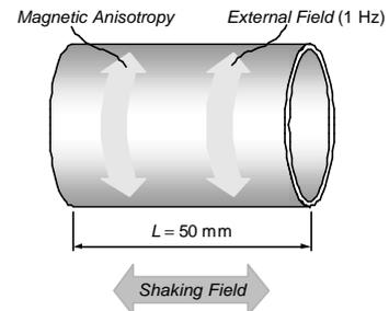
Fig. 5. Permeability measurement: the applied fields and magnetic anisotropy arrangement imitate the case of axial shielding. Low-frequency, 1 Hz, external field was applied by a toroidal coil wound around the shield. Magnetic induction was measured by another, separate toroidal coil. High-frequency, 1 kHz, shaking field was applied by a solenoid. Field magnitudes correspond to those used for measuring the axial shielding factor (Table. II).
