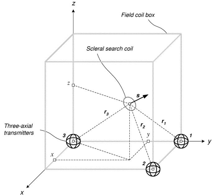
Fig. 3. Eye location tracking with a triad of three-axial transmitters. Finding the distances  $r_1, r_2, r_3$  between the three-axial transmitters and the SSC allows calculation of the eye location by applying the triangulation technique.
