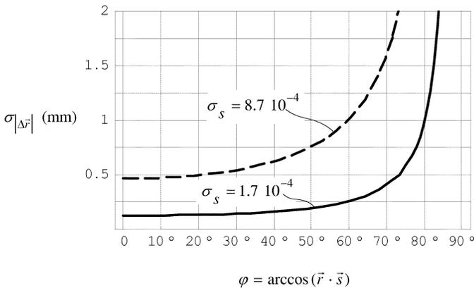
Fig. 2. The location resolution  $\sigma_{|\Delta\vec{r}|}$  as a function of the angle  $\varphi$  between the  $\vec{r}$  and  $\vec{s}$  vectors. The SSC is located at a 1-m distance from the transmitter, such that  $\vec{r} = (\sqrt{1/3}, \sqrt{1/3}, \sqrt{1/3})$ .
