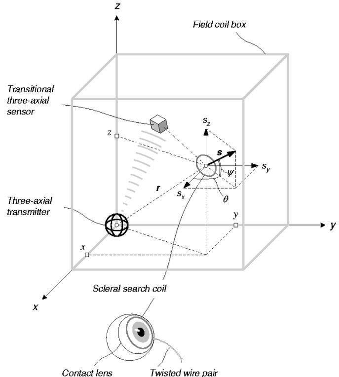
Fig. 1. A typical SSC system. To track the eye location, a conventional magnetic tracker consisting of the three-axial transmitter and the *transitional* three-axial magnetic sensor is added to the system. The three-axial transmitter is located outside the field coil box, and the transitional sensor is attached to the subject's head. The eye location,  $\vec{r} = (x, y, z)$ , is calculated *indirectly*, relative to the measured location and orientation of the transitional magnetic sensor.
