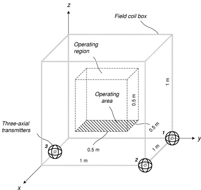
Fig. 5. Eye location tracking with a symmetrical triad of three-axial transmitters.
