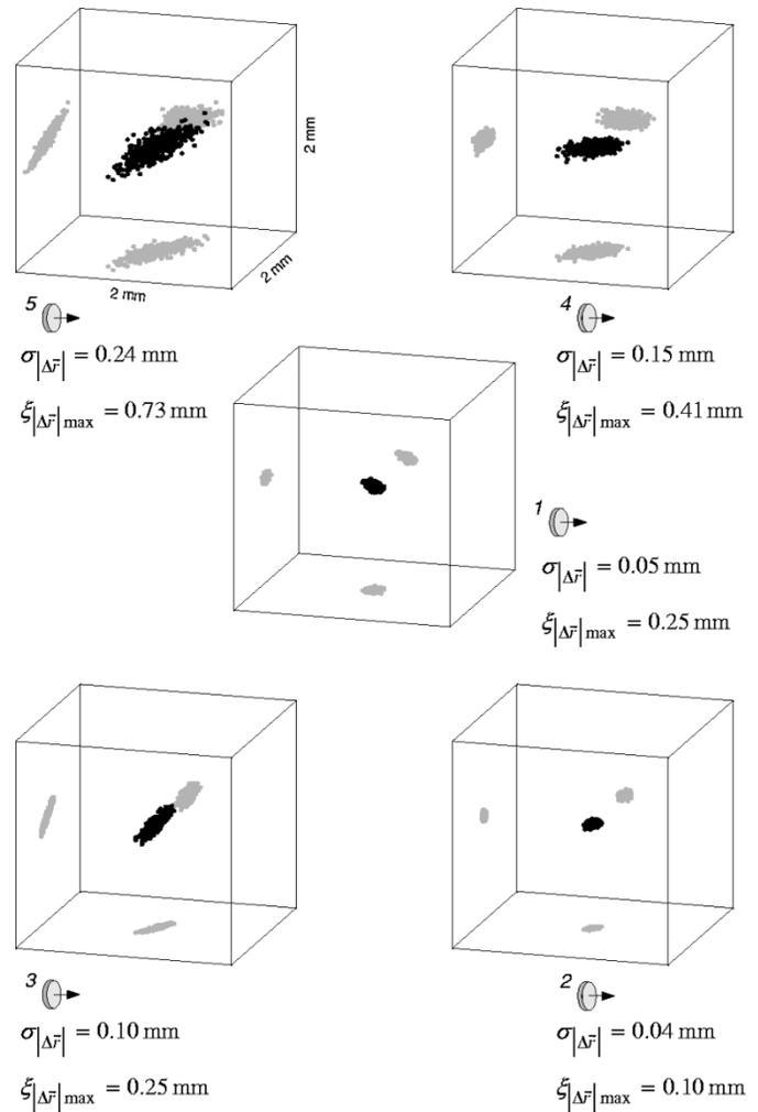
Fig. 8. Simulation of the SSC's location estimates for a  $\sigma_{H_s} = 10^{-4}$ ,  $\sigma_\theta = \sigma_\psi = 0.01^\circ$ . The SSC is situated in various locations throughout the operating region (see Fig. 7). Each cube corresponds to a  $2 \times 2 \times 2$  mm space around the true SSC's location. The black dots within the cubes represent the location estimates (500 total for each cube). The gray dots on the cubes' facets are projections (shadows) of the dots within the cube.
