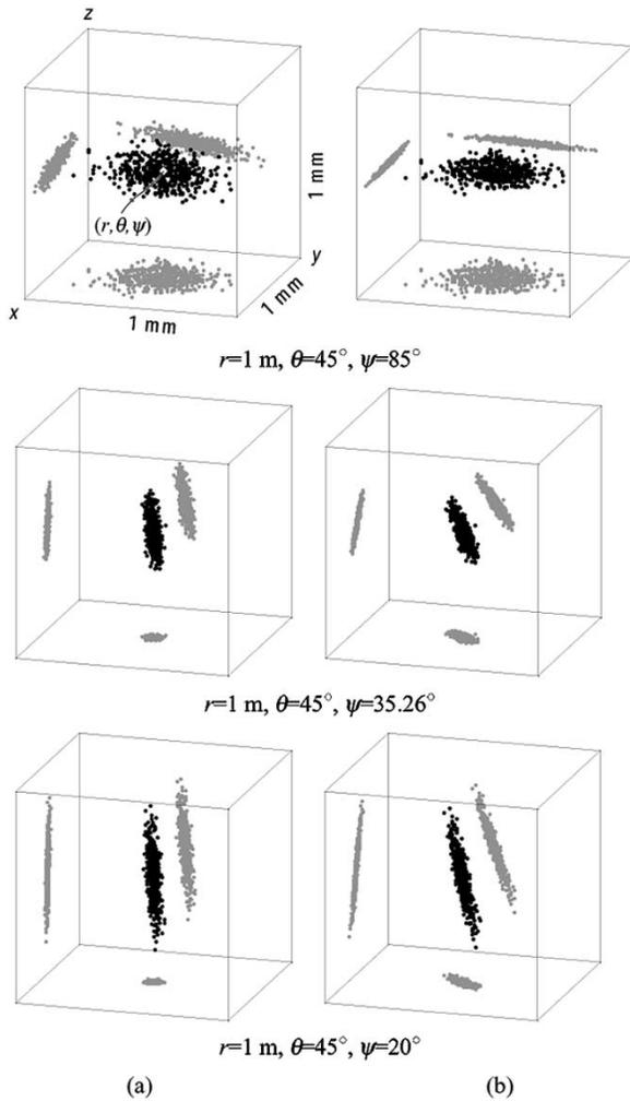
Fig. 5. Simulation of the sensor's location estimates for  $r = 1$  m,  $\theta = 45^\circ$  and different  $\psi$  under noise conditions  $\sigma_n = 10^{-5}$  (a) according to (3) and (b) according to (4). Each cube corresponds to a  $1 \times 1 \times 1$  mm area around the true sensor's location. The black dots within the cubes are the location estimations (500 total for each cube). The gray dots on the cubes' facets are projections of the dots within the cube.
