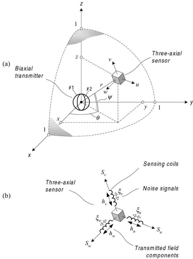
Fig. 3. Magnetic sensor location and structure. (a) Magnetic sensor is located at a fixed distance  $r = 1$  m from the transmitter. Note that  $z = \sqrt{1 - x^2 - y^2}$ . (b) Independent noise signals  $\xi_v, \xi_u, \xi_w$  are superimposed on the corresponding sensor vector outputs  $S_v, S_u, S_w$ .
