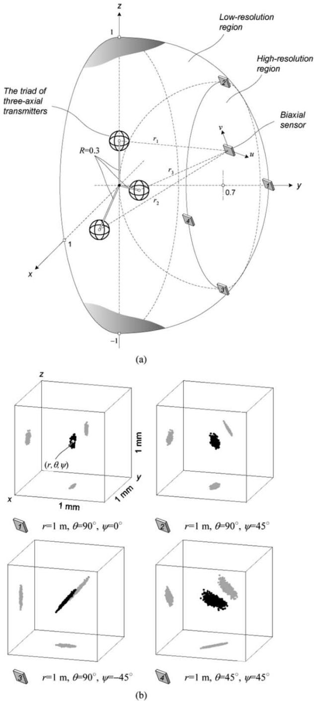
Fig. 7. Magnetic tracking with a triad of transmitters. (a) Magnetic sensor is located at a fixed distance  $r = 1$  m from the triad of transmitters. (b) Simulation of the sensor's location estimates under noise conditions  $\sigma_n = 10^{-5}$ . Each cube corresponds to a  $1 \times 1 \times 1$  mm area around the true sensor's location. The dots within the cubes are the location estimates (500 dots total for each cube).
