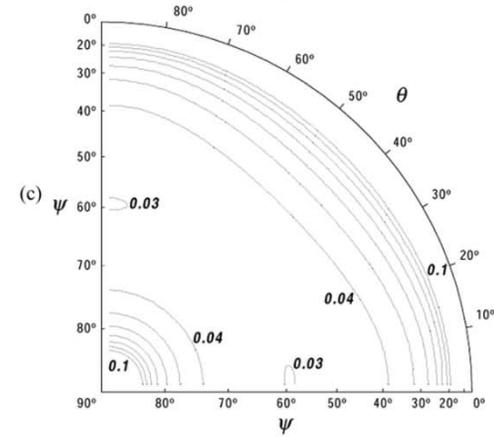
Fig. 4. Location resolution  $\sigma_{(x,y,z)}$  calculated for the sensor in Fig. 3(a) as a function of the sensor's coordinates  $x$  and  $y$  in (a) and as a function of  $\theta$  and  $\psi$  (contour plots) for method [3] in (b) and method [4] in (c). The bold numbers in parts (b) and (c) represent the location resolution,  $\sigma_{(x,y,z)}$ , measured in millimeters.
