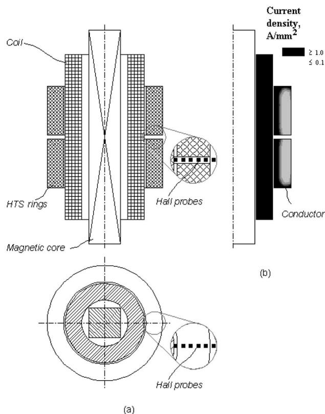
FIG. 1. (a) Experimental setup; (b) distribution of current in the almost perfect ( $10^{10}$  S/m) conductive ring (numerical simulation for 1 A/mm<sup>2</sup> primary current density and 50 Hz frequency).
