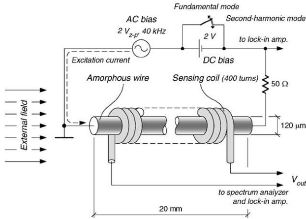
Fig. 1. Orthogonal fluxgate employing an amorphous wire.
