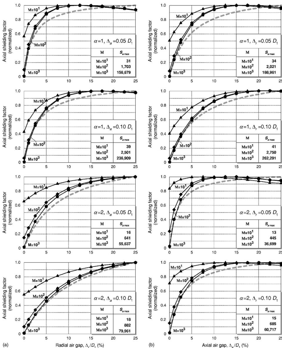
FIG. 4. The effect of the (a) radial and (b) axial air gap on the axial shielding factor for shields having different aspect ratios ( $\alpha=1$  and  $\alpha=2$ ), different axial air gaps ( $\Delta_a=5\%$  and  $10\%$  of  $D_1$ ), and different normalized permeabilities ( $M=10^1, 10^2$ , and  $10^3$ ). The dashed lines represent the approximation with Eq. (2).
