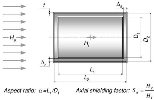
FIG. 2. Double-shell axial magnetic shield.
