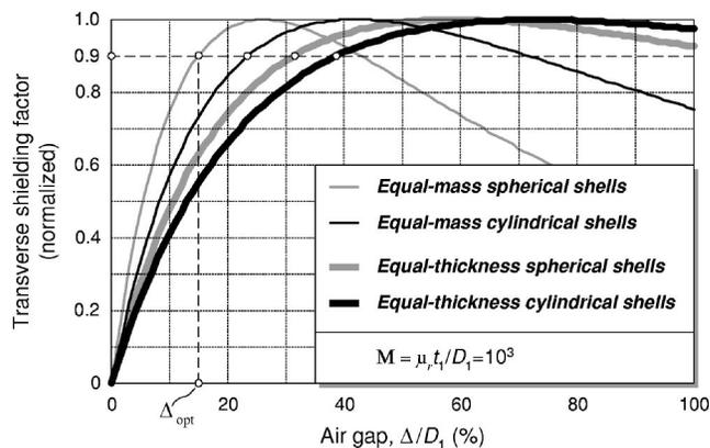
FIG. 1. The effect of the air gap  $\Delta = (D_2 - D_1)/2$  on the shielding with double-shell spherical and infinitely long cylindrical magnetic shields. Equal-mass shields provide the most effective shielding per unit mass, but most practical shields are made using constant thickness material.
