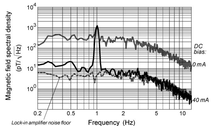
Fig. 5. Fluxgate noise spectra referred to the input. A 7-nT rms sinusoidal external magnetic field is applied to the fluxgate at a 1-Hz frequency. Note that the noise in the fundamental mode is by an order of magnitude lower than in the second-harmonic mode (BMH window, 12.5/400 linewidth).
