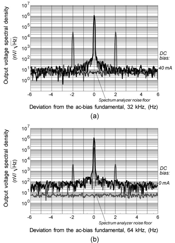
Fig. 4. Fluxgate resolution: the signal and noise (a) near the fundamental and (b) near the second harmonic. The gray line represent the case where a 7-nT rms sinusoidal external magnetic field is applied to the fluxgate at a 2-Hz frequency (BMH window, 12.5/400 linewidth).
