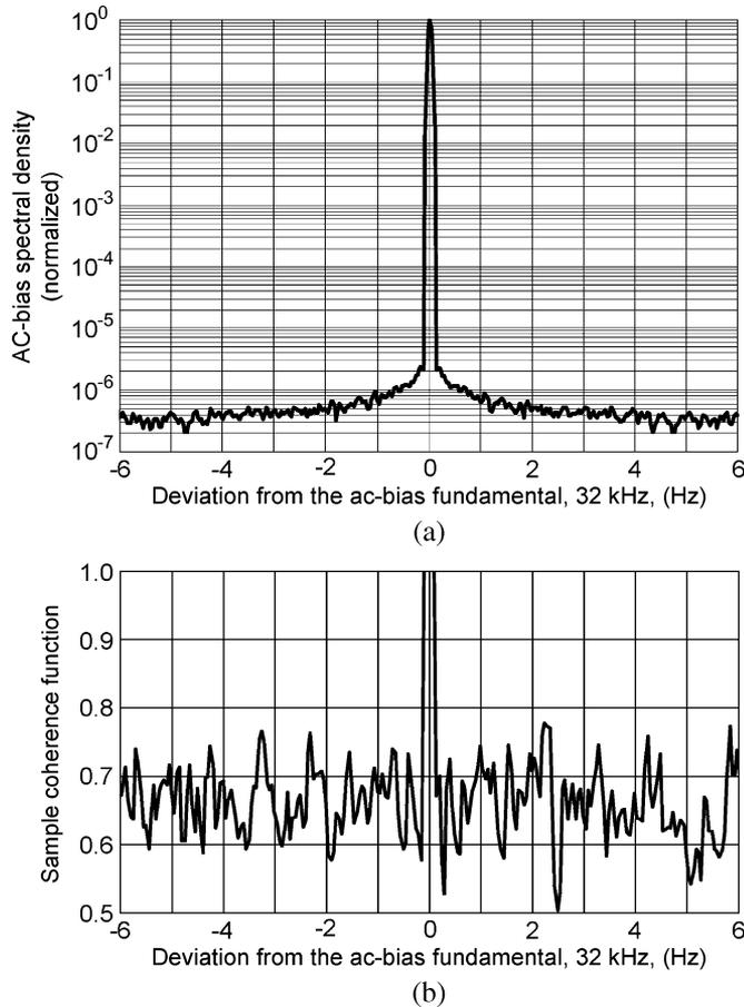
Fig. 6. Correlation between the noise of the fluxgate and the excitation. (a) Normalized amplitude spectrum of the excitation current (BMH window, 12.5/400 linewidth). (b) Sample coherence function of the fluxgate noise in the fundamental mode [see Fig. 4(a)] and the phase noise of the excitation in (a) (BMH window, 12.5/250 linewidth).
