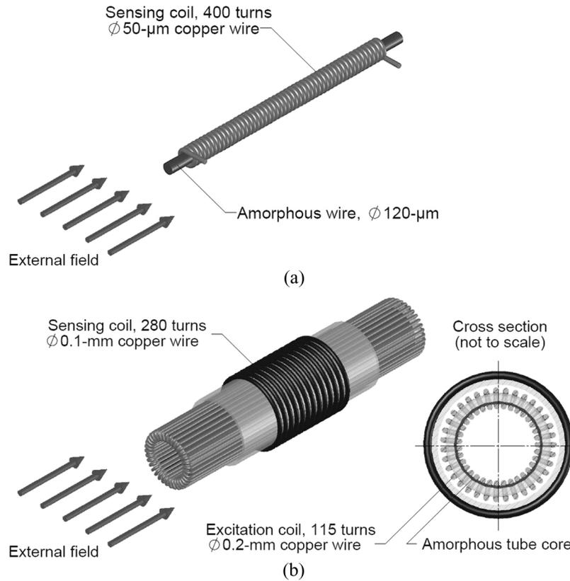
Fig. 1. Orthogonal fluxgates: (a) with amorphous wire core and (b) with tube core.
