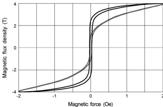
Fig. 2. DC hysteresis loops of the Metglas 2705M amorphous ribbon measured along (the black lines) and across (the gray lines) the ribbon length. The loop shapes reveal well-defined uniaxial anisotropy pointing along the ribbon length.
