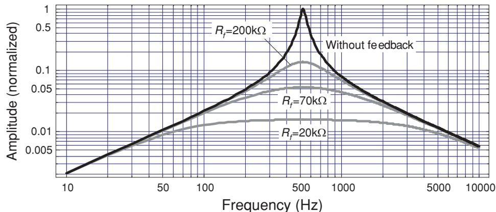
FIG. 6. (Color online) Magnetometer frequency response.
