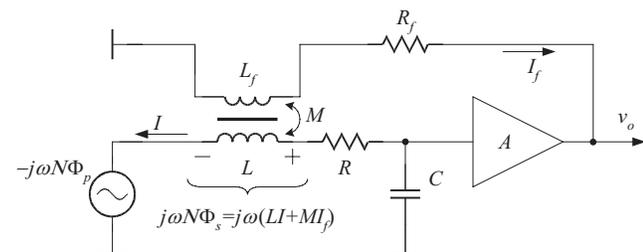
FIG. 2. Equivalent electrical circuit of the longitudinal magnetometer channel.
