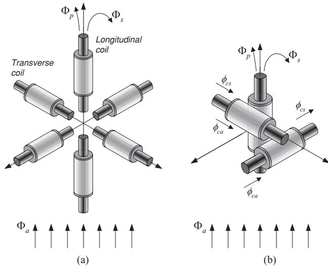
FIG. 1. Three-axial induction magnetometers: (a) a crosstalk free configuration, (b) a configuration with a crosstalk between the magnetometer coils.  $\Phi_p$  and  $\Phi_s$  are the primary and secondary fluxes in the longitudinal coil.  $\phi_{ca}$  and  $\phi_{cs}$  are the crosstalk components due to the applied,  $\Phi_a$ , and secondary fluxes, respectively.
