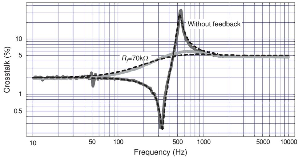
FIG. 10. (Color online) Total magnetometer crosstalk  $\phi_{c\Sigma}$ : a comparison between the theory and the experiment. The dashed and solid curves represent the theoretical and experimental data, respectively.
