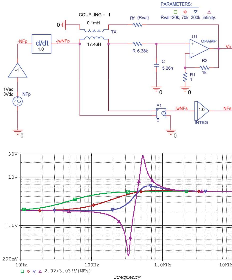
FIG. 12. (Color online) Crosstalk simulation in SPICE: (top) design schematic, (bottom) the total crosstalk  $\phi_{c\Sigma}$  as a function of frequency and the amount of feedback (volts correspond to %). (The letter “F” stands for “ $\Phi$ ”).
