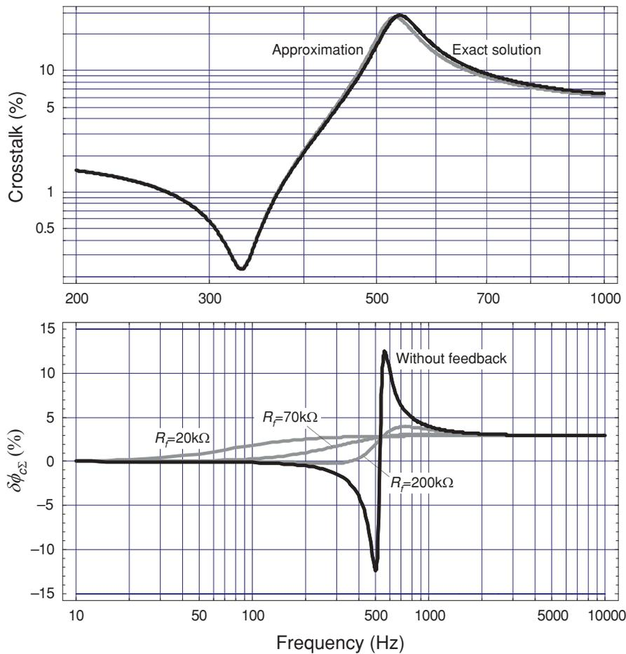
FIG. 11. (Color online) Exact and approximate crosstalk: (top) a comparison of the crosstalk values for the case of no magnetic feedback, (bottom) the relative error of the approximation.
