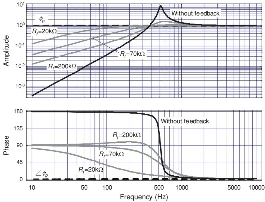
FIG. 7. (Color online) The secondary relative flux  $\phi_s$  as a function of frequency and the amount of feedback.
