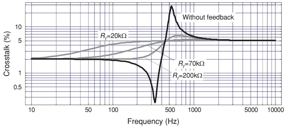
FIG. 9. (Color online) The total crosstalk  $\phi_{c\Sigma}$  as a function of frequency and the amount of feedback.
