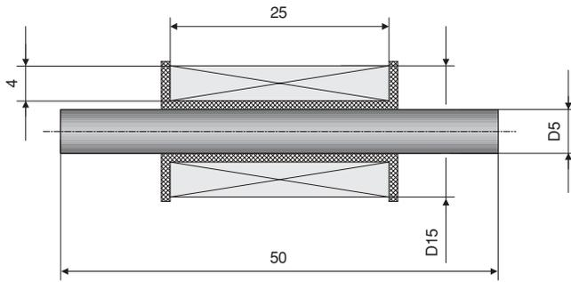
FIG. 5. Magnetometer coil.
