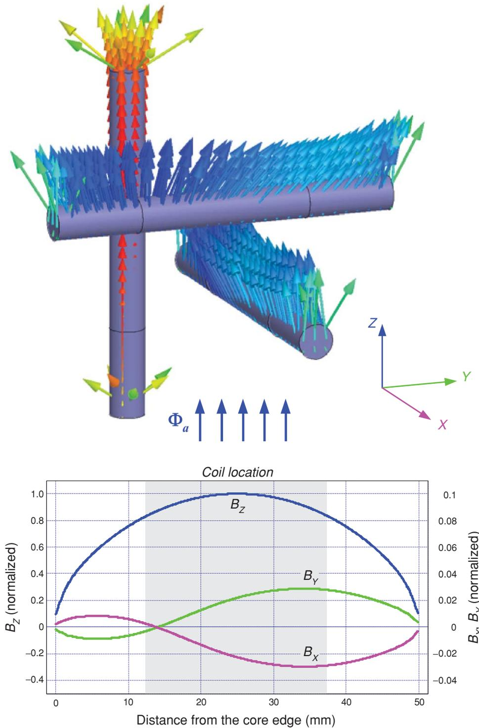
FIG. 3. (Color online) Crosstalk due to the applied flux  $\Phi_a$  (a uniform magnetic field is applied along Z-core): (top) magnetic induction within the cores, (bottom) magnetic induction along the core axes. The coils are not shown. Note that there are net magnetic fluxes within the transverse cores. Relative to the primary flux in the longitudinal coil, the crosstalk  $\phi_{ca1} = 2.02\%$ . The coil dimensions are given in Fig. 5. (Calculated with Maxwell 13.0.)
