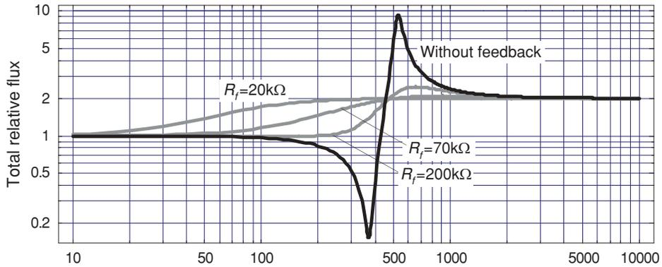
FIG. 8. (Color online) The total relative flux  $\phi_\Sigma$  as a function of frequency and the amount of feedback.
