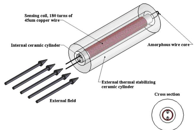
FIG. 1. (Color online) Orthogonal fluxgate employing an amorphous wire.
