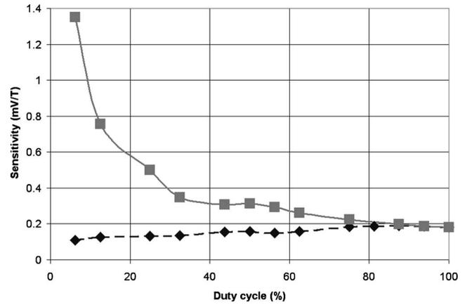
FIG. 3. Fluxgate sensitivity as a function of excitation duty cycle. The dashed curve represents the fluxgate sensitivity without eliminating the data related to the idle excitation intervals [see Fig. 2(b)]. The solid curve represents the fluxgate sensitivity after omitting the data related to the excitation idle intervals [see Fig. 2(c)].
