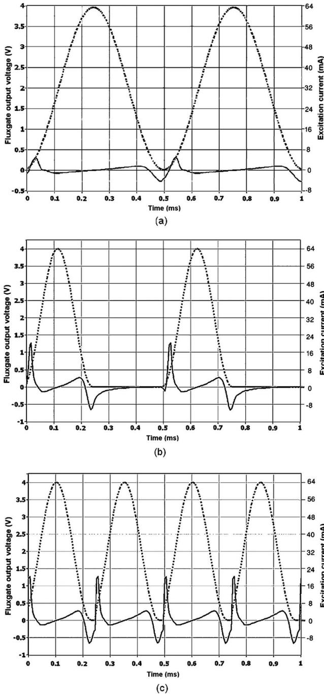
FIG. 2. Fluxgate output signal (the solid curves) and the excitation current (the dashed curves) in different excitation modes. (a) Continuous excitation (100% duty cycle). (b) Discontinuous excitation (50% duty cycle). (c) Discontinuous excitation (50% duty cycle) after discarding the data related to the idle intervals.
