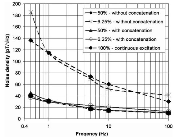
FIG. 5. Spectrum of the fluxgate noise referred to the fluxgate input.
