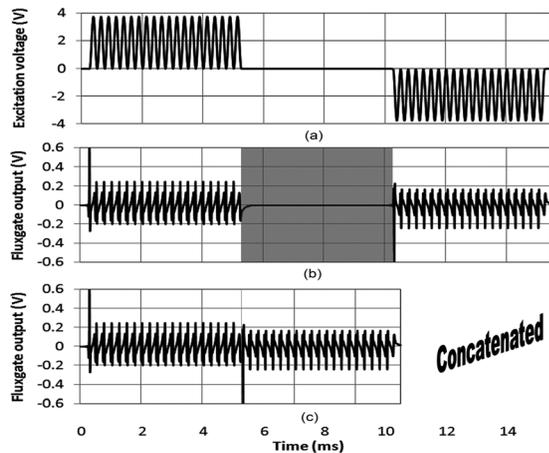
FIG. 6. Excitation with idle intervals between the dc bias reversals: the excitation waveform (a) and the fluxgate output (b). The signal parts shaded by gray ( $10t$  segments in this example) were eliminated from the fluxgate output and the remaining signal parts were concatenated (c).
