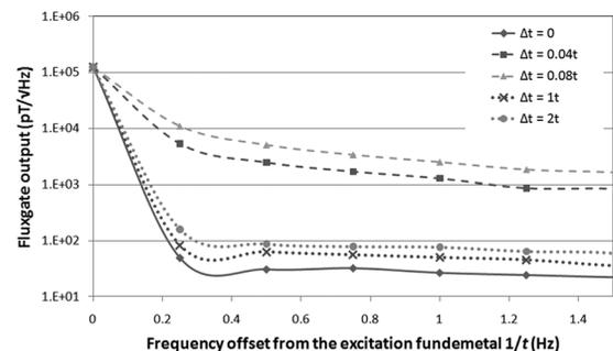
FIG. 5. Amplitude spectral density of the fluxgate output as a function of the sampling window duration: even very small deviations  $\Delta t$  of the sampling window duration from its spectral-leakage-free value of  $400T$  (see Fig. 4) cause significant increase in the floor of the fluxgate output spectrum (dashed curves). Deviations from  $T$  in the multiplications of  $t$  appear as dotted curves.
