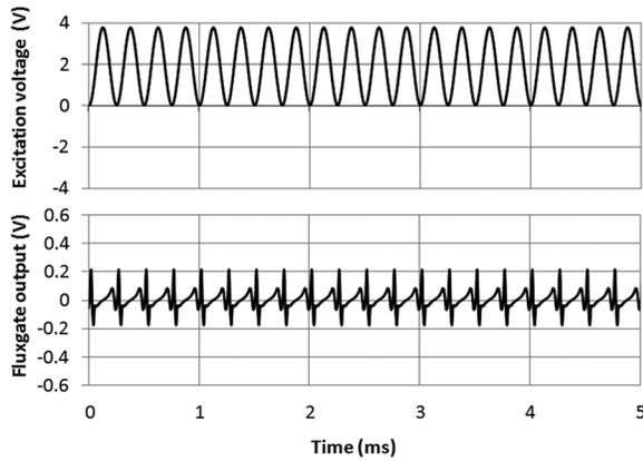
FIG. 2. Excitation with a constant dc bias: the excitation waveform (top) and the fluxgate output (bottom). The dc bias has a 1.9 V magnitude, and the ac excitation part has a 1.9 V amplitude and a 4 kHz frequency (0.25 ms period).
