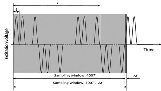
FIG. 4. Duration of the fluxgate output sampling window as compared to the excitation waveform:  $t$  is the period of the ac excitation cycle,  $T$  is the period of the alternating dc bias, and  $\Delta t$  is the deviation of the sampling window duration causing spectral leakage.
