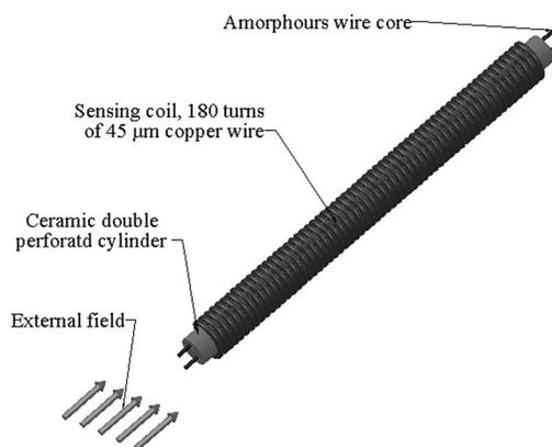
FIG. 1. Orthogonal fluxgate employing an amorphous wire.
