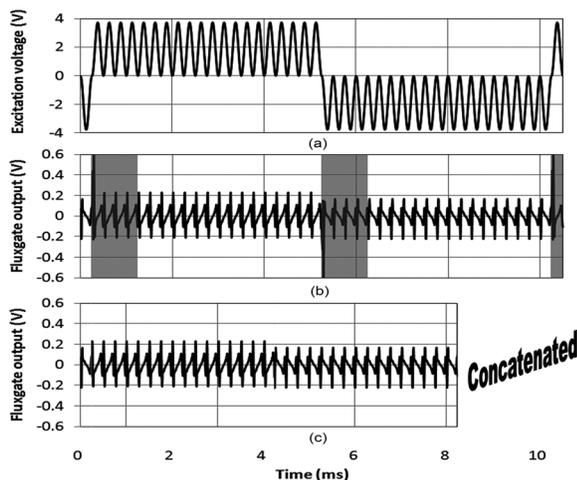
FIG. 3. Excitation with alternating dc bias: the excitation waveform (a) and the fluxgate output (b). Compared to Fig. 2, the dc bias reverses its polarity every  $T = 20t$  excitation cycles. The signal parts shaded by gray ( $4t$  segments in this example) were omitted from the fluxgate output and the remaining parts were concatenated (c).
