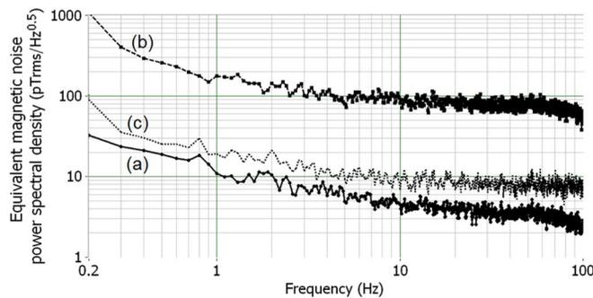
Fig. 5. Noise spectrum of the orthogonal fluxgate with (a) digital selective bandpass sampling with the lowest equivalent magnetic noise (sample #9 in Fig. 4), (b) sampling point with the highest equivalent magnetic noise (sample #20 in Fig. 4), and (c) the conventional sampling method.
