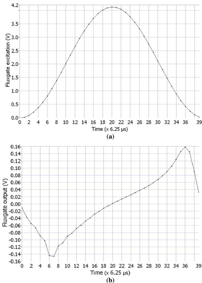
Fig. 2. Fluxgate excitation voltage (a) and the output signal (b).
