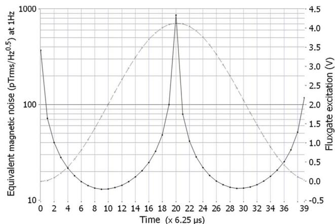
Fig. 4. Fluxgate equivalent magnetic noise (the solid curve) as a function of the sampling instances within the excitation cycle (the dashed curve).
