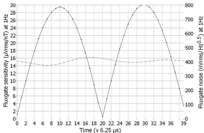
Fig. 3. Fluxgate output noise (the dashed curve) and sensitivity (the solid curve) as a function of the sampling instances within the excitation cycle.
