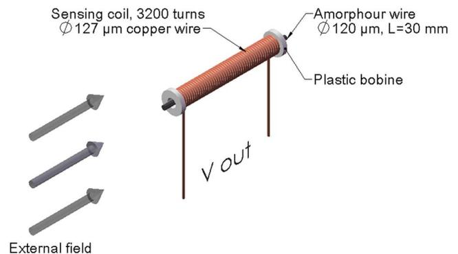
Fig. 1. Orthogonal fluxgate employing an amorphous wire.
