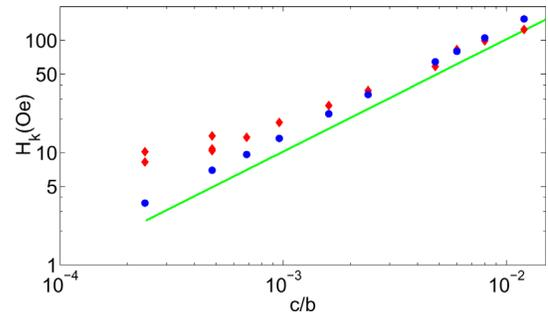
FIG. 4. (Color online) The experimental (diamonds) and simulated (dots) shape anisotropy field for ellipses as a function of the axes ratio  $b/c$ . The line represents the theoretical anisotropy field of ellipsoids [Eq. (8)].
