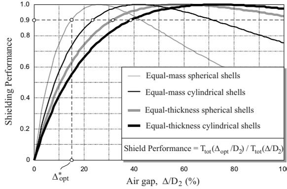
Figure 12.2 The effect of the relative air gap  $\Delta/D_2$  on the shielding performance of double-shell spherical and infinitely long cylindrical ferromagnetic shields.
