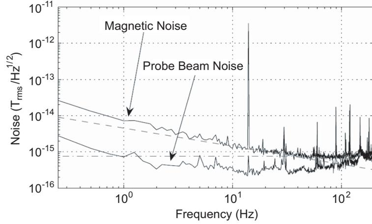
Figure 12.5 Magnetic-field noise from the Princeton ferrite shield [33]. The dashed line represents noise of  $4.4 f^{-1/2}$  fT where  $f$  is in Hz. In comparison, white noise from a Mumetal shield of the same size was estimated to be  $18 \text{ fT}/\text{Hz}^{1/2}$ .
