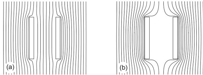
Figure 12.6 Magnetic field lines around an open superconducting cylinder. (a) Field was applied before the cylinder became superconducting. (b) Field was applied after the superconducting transition.
