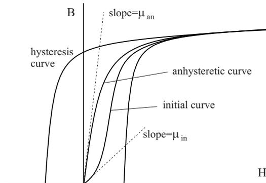
Figure 12.3 Hysteresis magnetization curve of a ferromagnetic material and various definitions of permeability.
