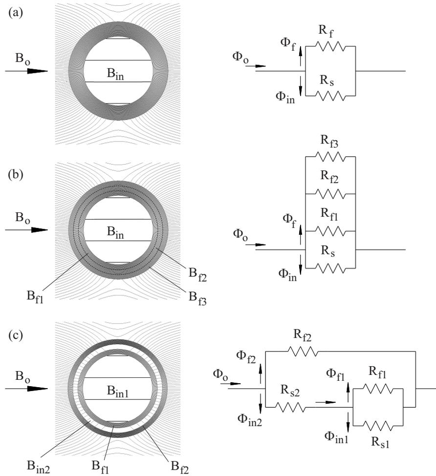
Figure 12.1 Magnetic circuit approach to estimating the performance of a multilayer shield.
