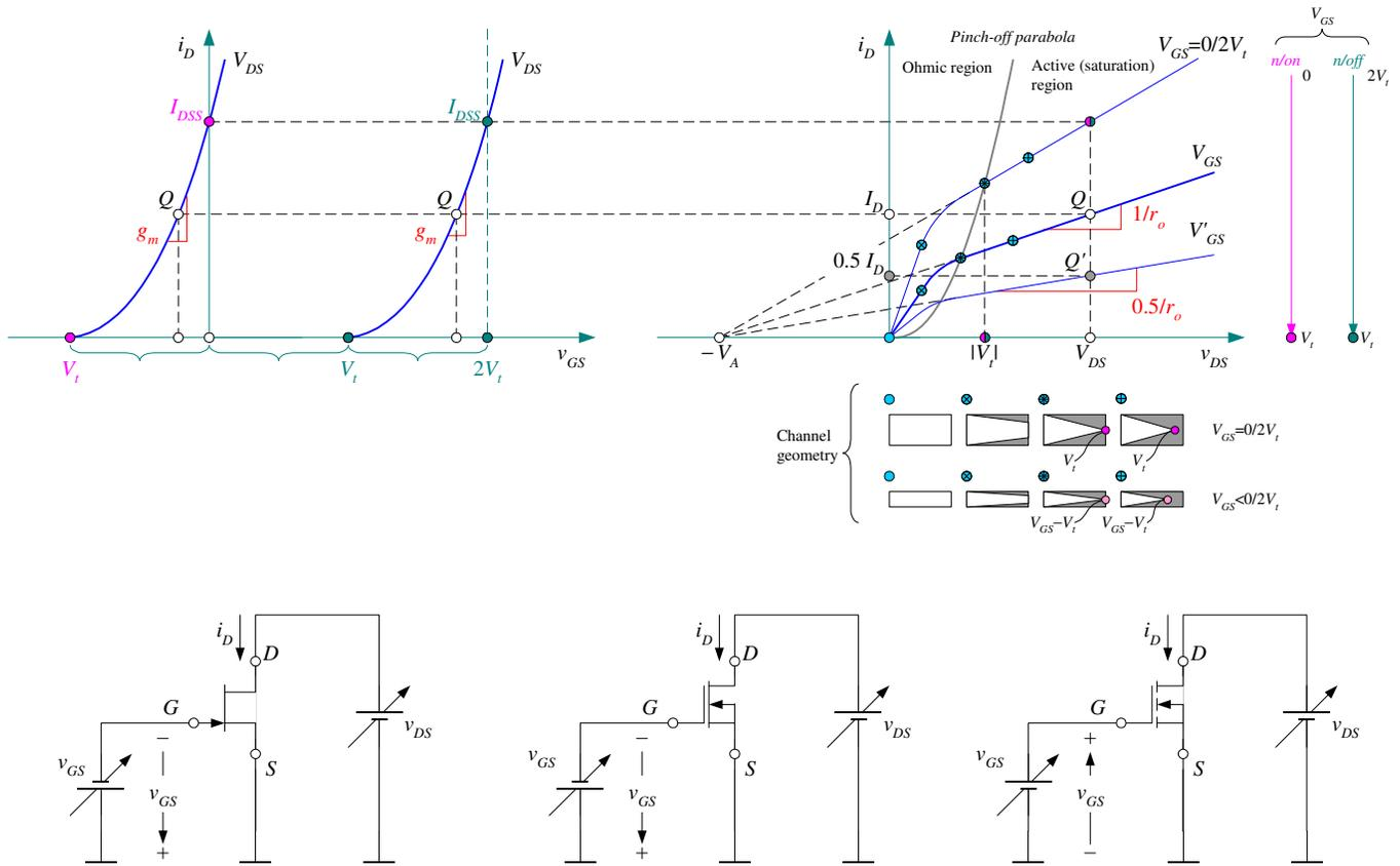
Fig. 2. Common-source characteristics of FET transistors.
