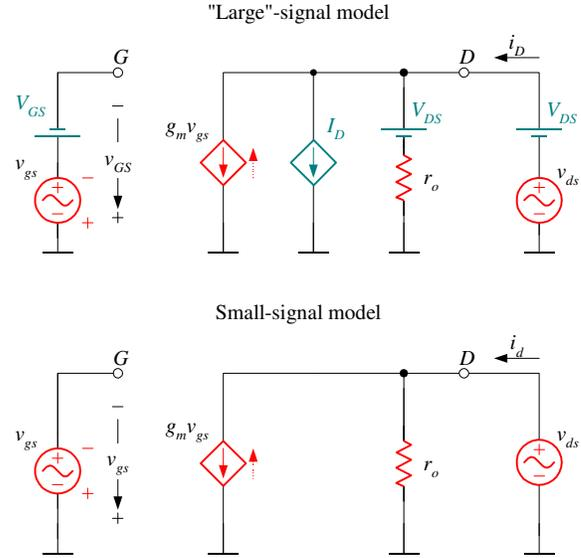
Fig. 3. "Large"- and small-signal models for the FET transistors. Note that the polarity of the small-signal source can be reversed and this will cause reversing the direction of the dependent current source  $g_m v_{gs}$ .
