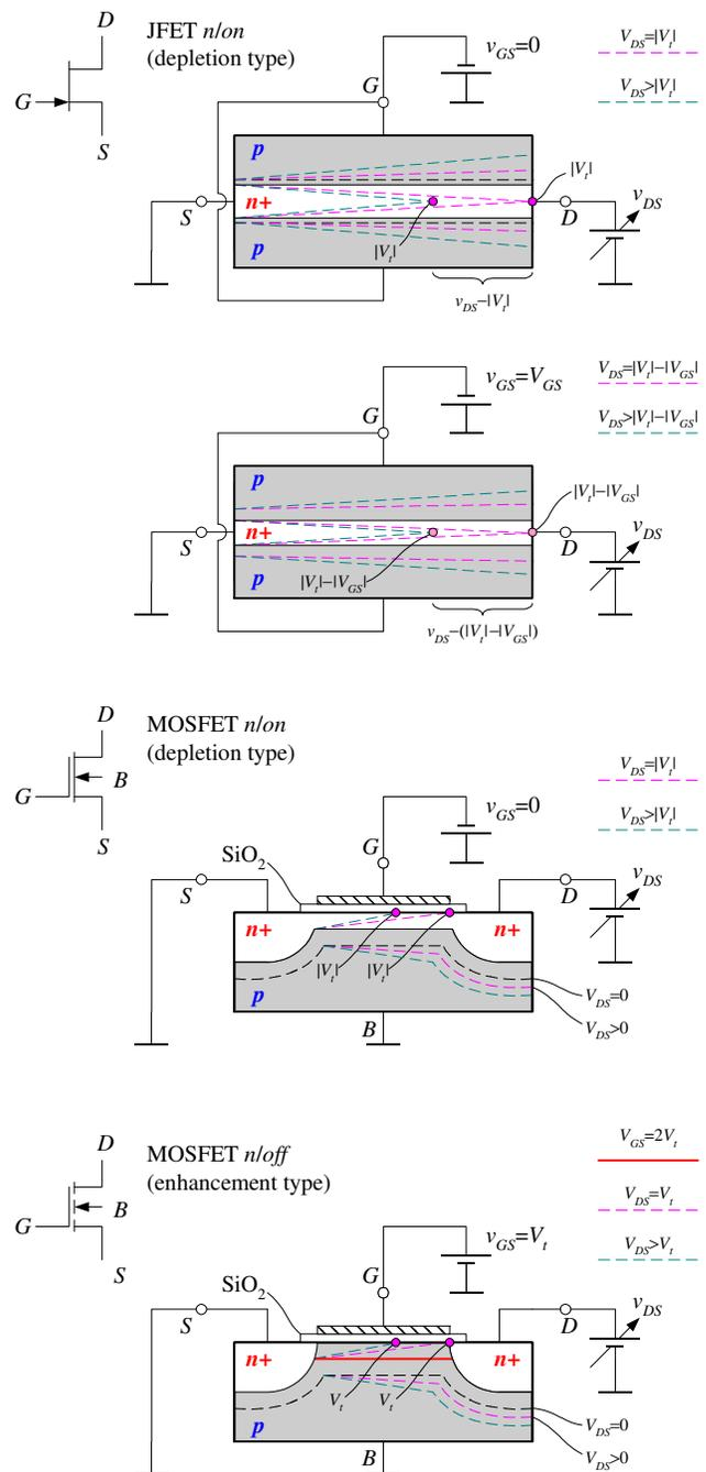
Fig. 1. The symbols of the JFET and MOSFET transistors (with the  $n$ -type channel) and their physical structures. For MOSFETs, the operation only at  $V_{GS}=0$  and  $V_{GS}=2V_t$  is shown for the  $n/on$  and  $n/off$  types, respectively. Note that for lower  $V_{GS}$ , the pinch-off voltage, for both the MOSFETs, will be  $V_p=V_{GS}-V_t$ , as shown for the JFET.
