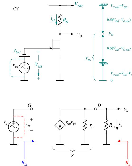
Fig. 5. Elementary CS amplifier: the static state and the equivalent small-signal circuit.
