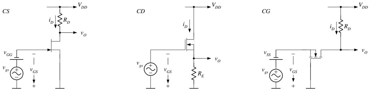
Fig. 4. Elementary single-transistor FET amplifiers.
