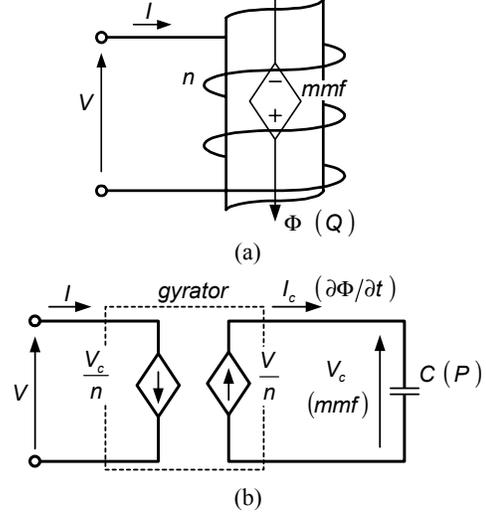
Fig. 1. A simple magnetic branch (a) and its equivalent gyrator-capacitor model (b).
