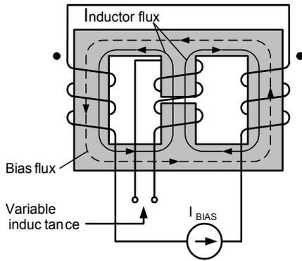
Fig. 4. Winding arrangements of the a current-controlled inductor [1].
