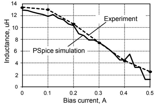
Fig. 6. Simulated and measured inductance of the current-controlled inductor versus bias current.
