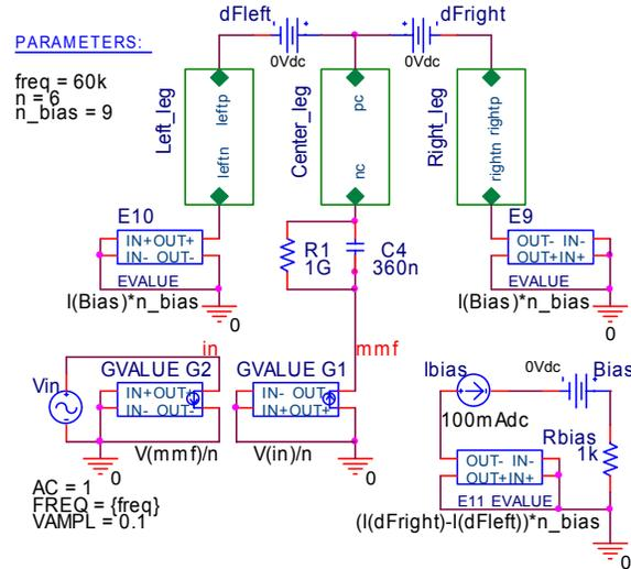
Fig. 5. PSPICE model of the current-controlled inductor of Fig. 4.
