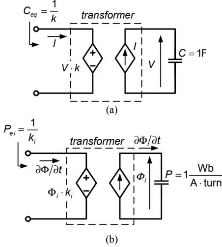
Fig. 2. A variable capacitor model (a) and its application to emulate a non-linear permeance (b).
