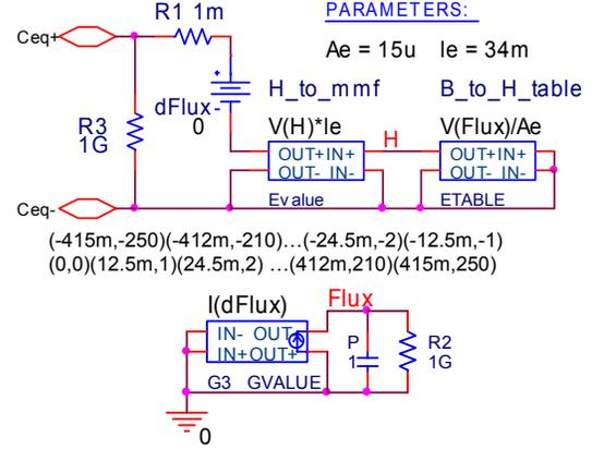
Fig. 3. PSPICE (CADENCE Eval. Version 9.2 ) model of non-linear capacitor, which emulates relationships between a magnetic flux  $\Phi$  (an electric charge of capacitor) and the mmf (the input terminals voltage). Branch parameters:  $A_e = 15\mu\text{m}^2$  and  $l_e = 34\text{mm}$ . Core material: 3F3 [5].
