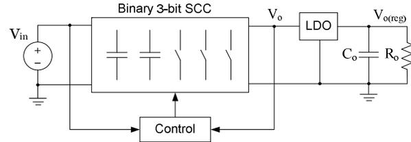
Fig. 9. Block diagram of output voltage regulation by LDO at the output.
