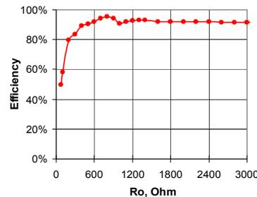
Fig. 15. Efficiency of step-up EXB based SCC,  $M_3 = 8/3$ .
