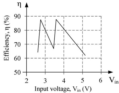
Fig. 3. The output characteristics of a commercial SCC [12] set to an output voltage of 1.8V.
