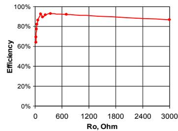
Fig. 14. Efficiency of step-down EXB based SCC,  $M_3 = 3/8$ .
