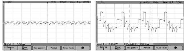
Fig. 13. Output ripple.  $V_{in}=8V$  and  $R_o = 437\Omega$ . (a)  $M_3 = 3/8$ . (b) Dithering between  $M_3 = 3/8$  and  $M_1 = 1/2$  (in 4:1 ratio). Vertical scale: 10mV/div; Horizontal scale: 100µs/div.
