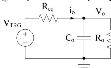
Fig. 2. The SCC equivalent circuit.
