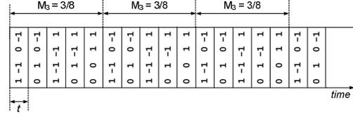
Fig. 7. SCC sequencing for  $M_3 = 3/8$ .
