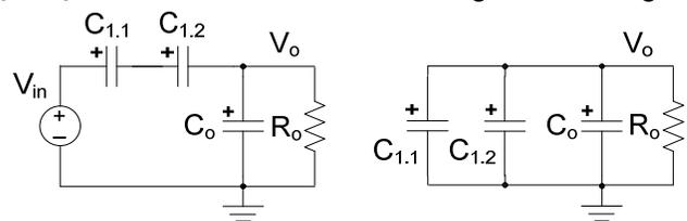
Fig. 5. Capacitors connections that follow the GFN codes of  $N_1(3) = 1/3$ .
