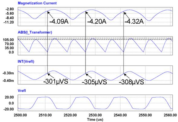
Fig. 8. Simulation results of the resonant converter of Fig. 6. Upper trace – transformer's magnetization current, second trace – rectified transformer primary current, third trace – 'Volt-seconds' of transformer's primary voltage, bottom trace – transformer's primary voltage.
