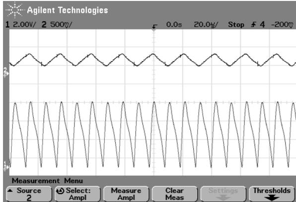
Fig. 12 Experimental results - unbalanced condition. Upper trace: Output of DC sensor, 2.27A/div; Lower trace: Rectified transformer's primary current, 20A/div, Horizontal scale 20µs/div.
