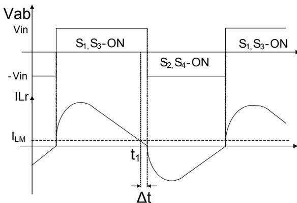
Fig. 5. Transformer primary current with none zero magnetization current.
