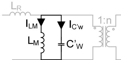
Fig. 10. Components that cause ripple current when primary and secondary currents are summed. Interwinding capacitance ( $C_W$ ) is reflected to primary ( $C'_W$ ).
