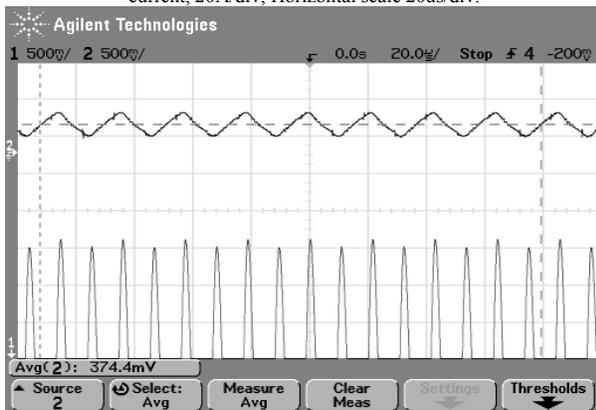
Fig. 13 Experimental results - unbalanced condition. Upper trace: Output of DC sensor, 2.27A/div; Lower trace: Rectified transformer's primary current (zoom of the corresponding trace in Fig. 12), 5A/div. Horizontal scale 20µs/div.
