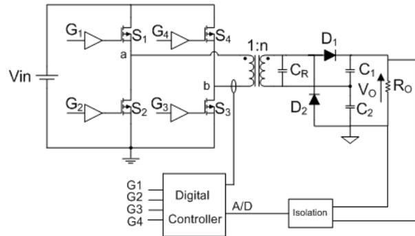
Fig. 1. The parallel resonant converter under consideration.
