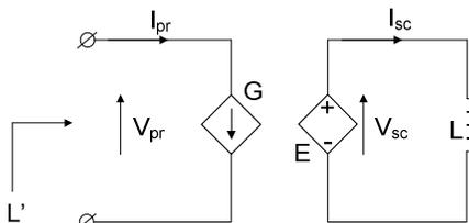
Fig. 7. Behavioral model of a non-linear inductor used in PSIM simulation. See text for definition of dependent sources.
