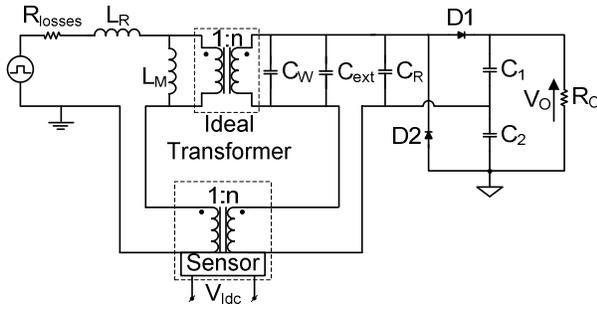
Fig. 9. Proposed method for measuring transformer's DC current.
