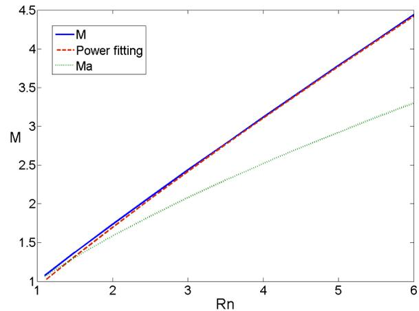
Fig. 4. Voltage transfer function  $M$ , approximate expression  $M_a$  and fitted curve "Power fitting"
