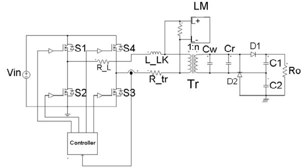
Fig. 6. PSIM simulation model used to explore the behavior of the resonant converter of Fig.1.
