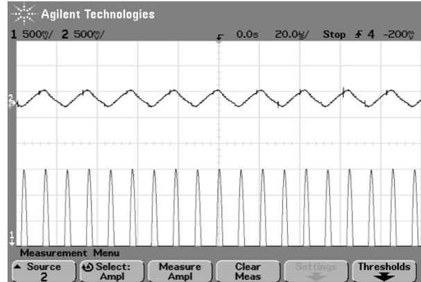
Fig. 15 Experimental results - near balanced condition. Upper trace: Output of DC sensor, 2.27A/div; Lower trace: Rectified transformer's primary current, 5A/div. No asymmetry detected. Horizontal scale 20µs/div.
