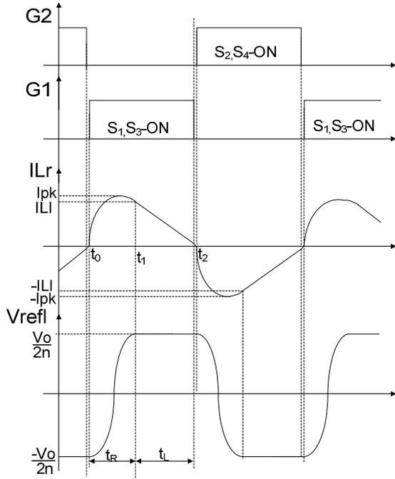
Fig. 2. Basic waveforms of the resonant converter of Fig. 1.  $I_{Lr}$  is the transformer's primary current,  $V_{refl}$  is the reflected voltage to transformers primary side.
