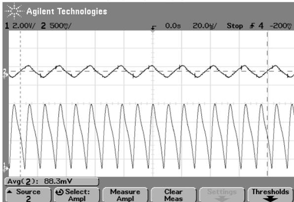
Fig. 14 Experimental results - near balanced condition. Upper trace: Output of DC sensor, 2.27A/div; Lower trace: Rectified transformer's primary current. Horizontal scale 20µs/div.
