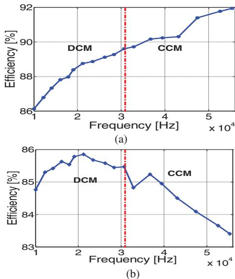
Fig.6: Conversion efficiency of proposed converter as a function of switching frequency for 0.5V input voltage and output power of about 1.2W. (a) Without considering gate drive losses. (b) Total efficiency when taking into account gate drive losses.
