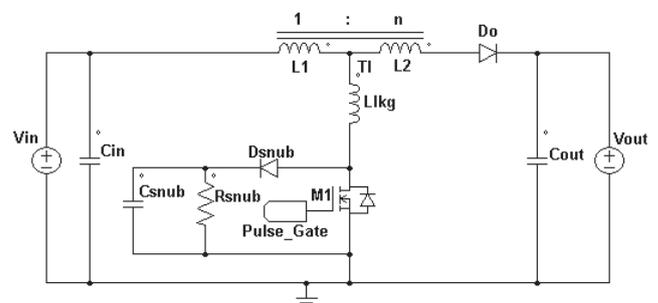
Fig. 1. Proposed high tapped-inductor boost ratio DC-DC converter
