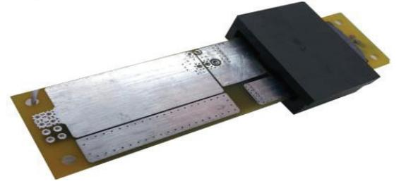
Fig.3. The assembled Flat Magnetics PCB
