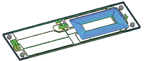
Fig.2. Design of the Flat Magnetics, PCB 2<sup>nd</sup> layer
