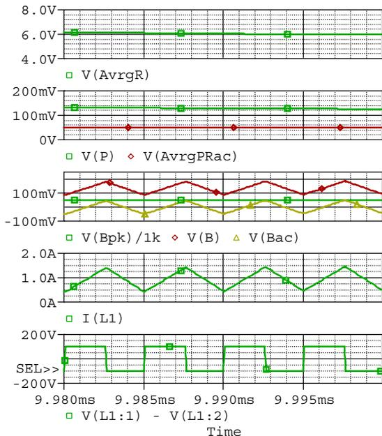
Fig. 4. Example of simulation output of Buck circuit. See Fig. 3 and Fig. 5 for definition of curves, and PARAMETERS in Fig. 3 for operating conditions. Ferrite material: 3F3.
