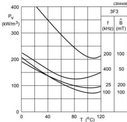
Fig. 2. Typical core loss temperature data given by manufacturers. (Ferroxcube, no endorsement implied)
