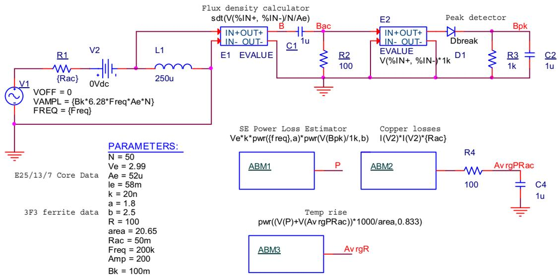
Fig. 3. Proposed model of ferrite core losses and hot spot temperature estimation.
