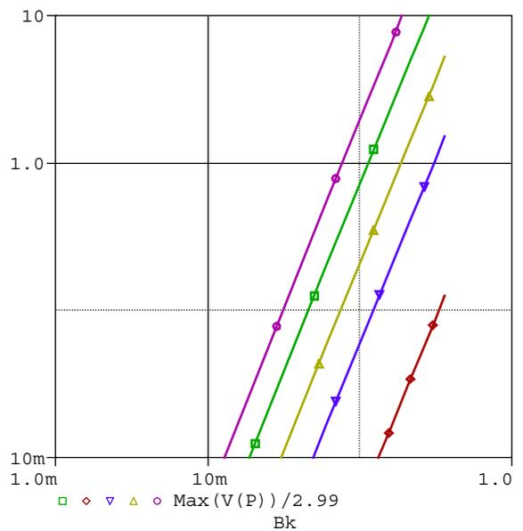
Fig. 5. Estimation of the average power loss of 3F3 E25/13/7 core by the simulation model of Fig. 3. (Compare to Fig. 1)
