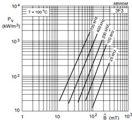
Fig. 1. Typical core loss data given by manufacturers. (Ferroxcube, no endorsement implied)
