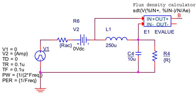
Fig. 5. Detail of Buck core loss simulation model. (The rest of the schematics is as in Fig. 3.)
