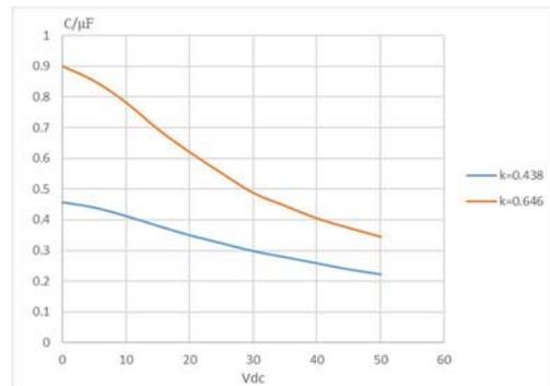
Fig. 7. Capacitance as a function of bias voltage of the ceramic capacitors assembly used in the  $k=0.646$  (upper curve) and  $k=0.438$  experiments.
