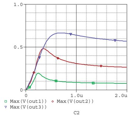
Fig.3. Simulation WPT voltage transfer function as a function of  $C_s$ .
