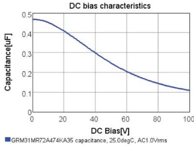
Fig. 4a. Incremental capacitance of GRM31MR72A474KA35 (Murata)
