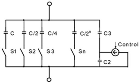
Fig 5. Proposed discrete/continuous controlled-capacitance assembly.
