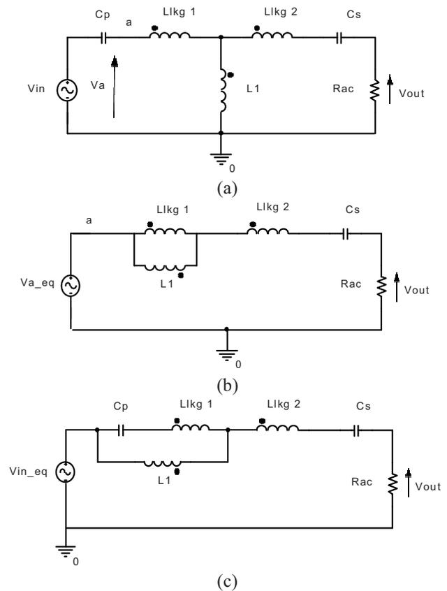
Fig. 1. Simplified Thevenin equivalent circuit model of a WPT system. (a) The transformer equivalent circuit. (b) Thevenin equivalent. (c) Taking primary capacitor  $C_p$  into account.
