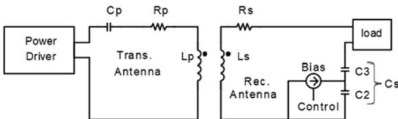
Fig. 2. Proposed variable capacitor controlled WPT system.
