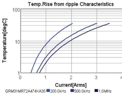
Fig.4b. Temperature rise and a function of current of CC of Fig. 4a.
