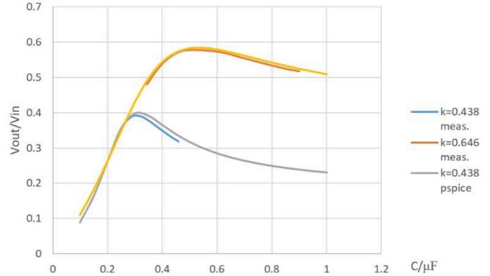
Fig. 9. Simulation and experimental results. Upper curves: k=0.646; Lower curves: k=0.438. Measured data are lower than simulated.
