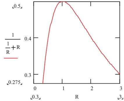
Fig. 4. Normalized output power as a function of R for  $Y=1$ ,  $V_{in}=1$  (equation 2).
