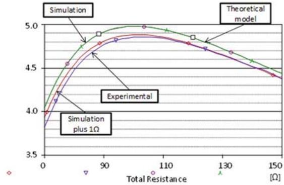
Fig. 8. Comparison of experimental, simulation and model calculation results. “Simulation plus 1Ω” accounts for parasitic resistance in experimental set up.
