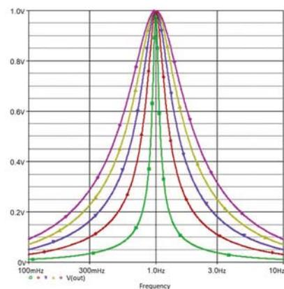
Fig. 2. Typical voltage gain ratio of a series resonant network for a range of load resistors.
