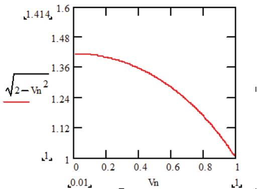
Fig. 6. Normalized output current  $I_n$  ( $I_n = I_o/I_{om}$ ), vertical axis, as a function of the normalized output voltage ( $V_n = V_o/V_{om}$ ) - per equation (9).
