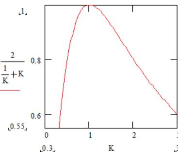
Fig. 5 Relative change in power as a function of relative change in load resistance (equation 6).
