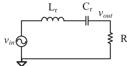
Fig. 1. The generic series resonant converter.
