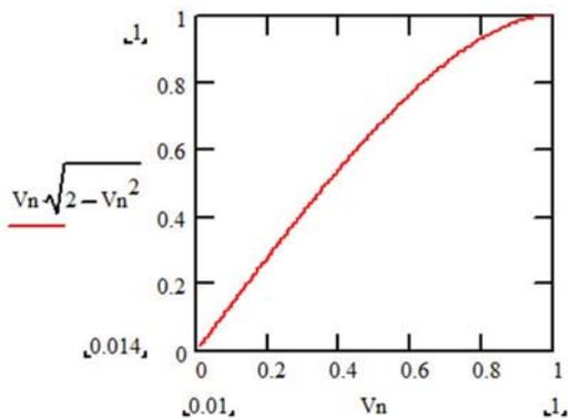
Fig. 7. Normalized output  $P_n$  ( $P_n = P_o/P_{om}$ ), vertical axis, as a function of the normalized output voltage ( $V_n = V_o/V_{om}$ ) - per equation (11)
