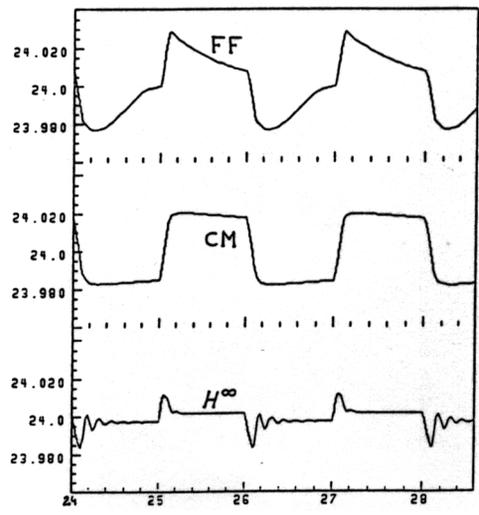
Fig. 5. The output voltage with rectangular perturbation in the input voltage, ±1V
