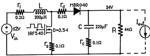
Fig. 1. The boost converter in the design example
