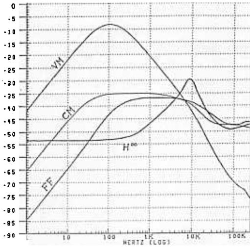
Fig. 3. The input to output voltage disturbance attenuation, in dB
