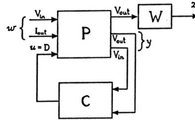
Fig. 2. The control of the converter as a standard  $H^\infty$  control problem
