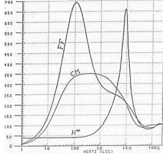
Fig. 4. The output impedance, in mΩ
