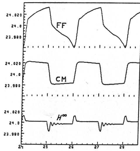
Fig. 6. The output voltage with rectangular perturbation in the load, ±50mA
