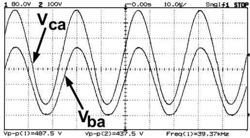
Fig. 16. Excitation voltage (upper trace) and voltage across a blocking direction switch (Fig. 11). Horizontal scale: 10 mSec/div. Vertical scale: 80 V/div, upper trace; 100 V/div, lower trace.
