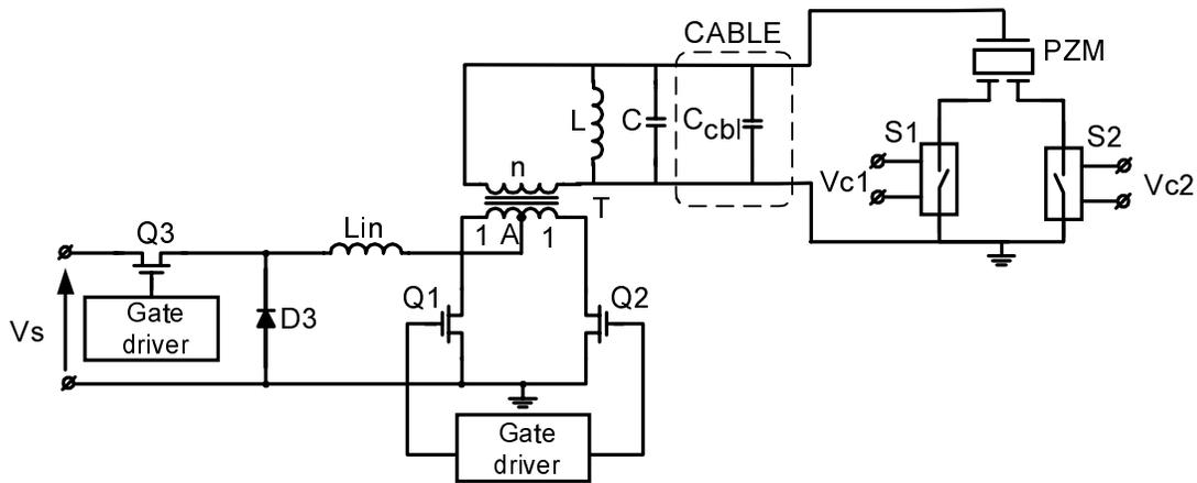
Fig. 6. Basic configuration of proposed PPRI driver.  $S_1$   $S_2$  control direction of motion (see Figs. 1 & 2).
