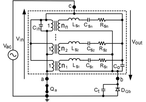
Fig. 12. Equivalent circuit of a PZM controlled by the direction switches of Fig. 11 when  $Q_a$  is 'on' and  $Q_b$  is 'off'.
