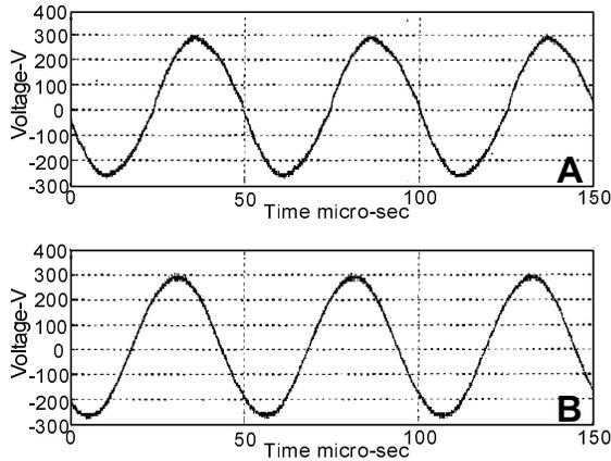
Fig. 13. PZM voltage when driven by proposed PPRI drive. (A) 3 m cable (0.6 nF). (B) 10 m cable (2 nF).
