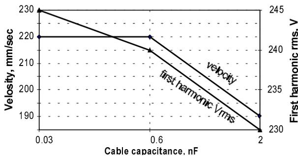
Fig. 14. PZM velocity and rms of first harmonics when driven by proposed PPRI driver, as a function of added capacitance.
