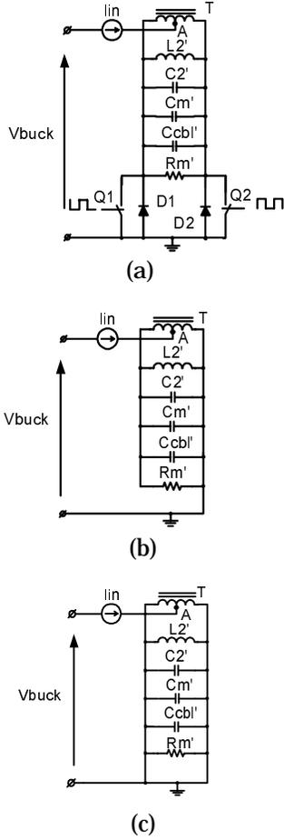
Fig. 7. Equivalent circuit of the PPRI driver (Fig. 6) with the secondary reflected to primary. (a) general circuit. (b) resonant mode. (c) boost mode.
