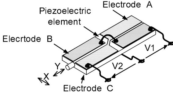
Fig. 1. Electrode configuration in a piezoelectric element of a PZM operating in longitudinal plus flexural mode (Nanomotion Ltd., Israel)
