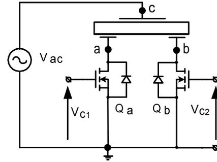
Fig. 11. Proposed single transistor direction switches.
