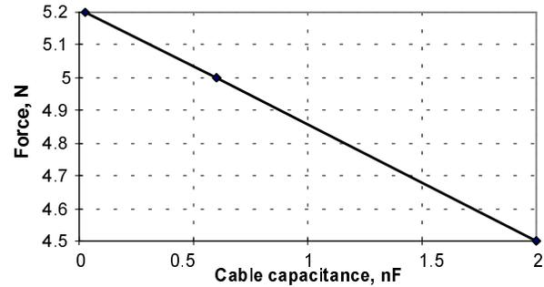
Fig. 15. PZM force when driven by proposed PPRI driver, as a function of added capacitance.
