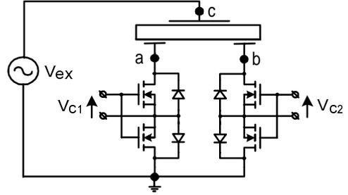
Fig. 10. Direction control by two transistors AC switched.
