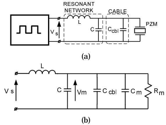
Fig. 4. LC type PZM driver. (a) system configuration. (b) equivalent circuit.
