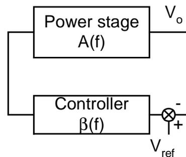
Fig. 4. Basic feedback loop in switch mode converters.
