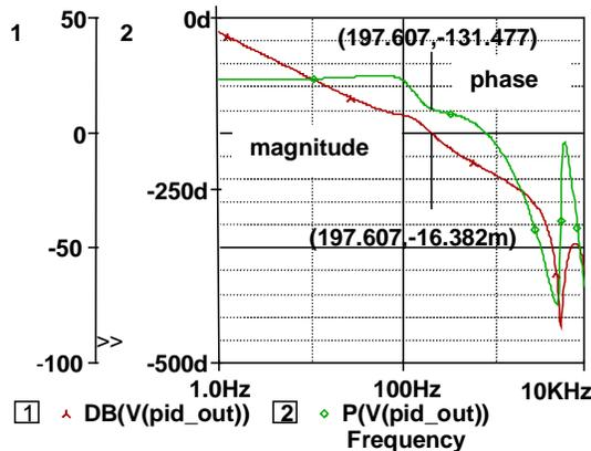
Fig. 12. Open loop frequency response of Boost converter with digital PID control as obtained by average simulation.
