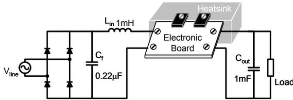
Fig. 10. Experimental set up.
