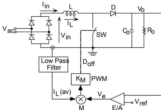
Fig. 3. Implementation of an APFC control scheme with no sensing of input voltage.
