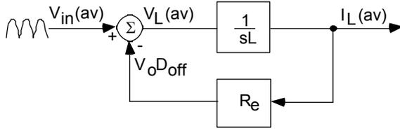
Fig. 5. Simplified block diagram of current control loop.
