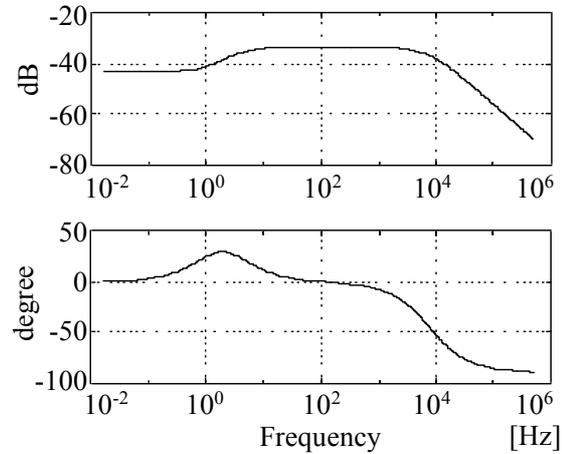
Fig. 7. Transfer function of the current control loop.
