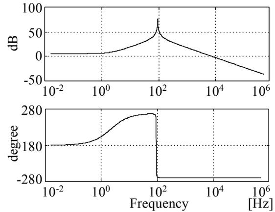
Fig. 6. Loop gain of the current control loop.
