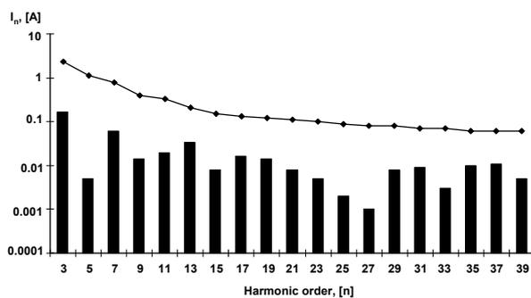
Fig. 12. Compliance with EN61000-3-2 standard at the 1kW level. Line: standard limits. Bars: measured harmonics. Notice the logarithmic scale.
