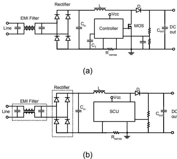
Fig. 9. Implementation of proposed control scheme is in a “discrete” form (a) and in an IC form (b).
