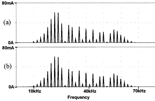
Fig. 4. Signal spectra. (a) Current in the original circuit [Fig. 2(a)]. (b) Reconstructed current spectrum. See text for details.
