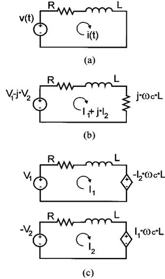
Fig. 2. SPICE model for a circuit with an "imaginary" resistor. (a) Original  $R$ ,  $L$  circuit driven by a modulated voltage source. (b) Equivalent circuit of (a) in the generalized phasor domain. (c) Cross-coupled equivalent circuits based on (11) and (12) that replace (b).
