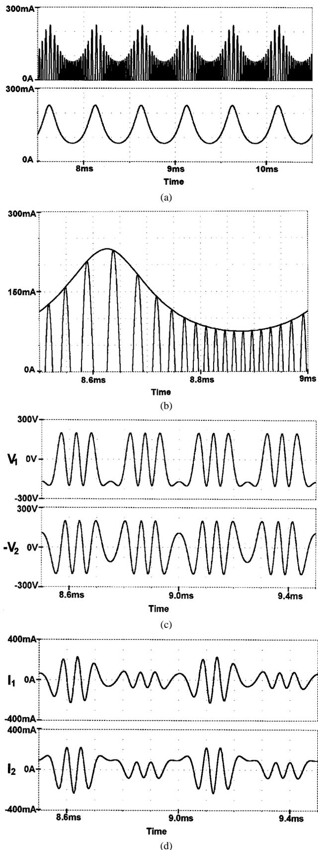
Fig. 3. Simulation results on the circuit of Fig. 2. (a) Current  $i$  through the original circuit of Fig. 2(a) (upper trace) and envelope of the current, obtained by envelope simulation based on Fig. 2(c) (lower trace). (b) Traces in (a) zoomed and superimposed. (c) Voltage phasor components  $V_1$  and  $-V_2$ . (d) Current phasor components  $I_1$  and  $I_2$ .
