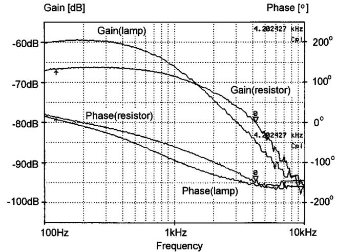
Fig. 8. Measured small-signal response of the experimental ballast (Fig. 6) loaded by a resistor (150 Ohm) and a fluorescent lamp load.
