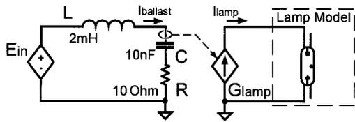
Fig. 11. Separated (tandem) scheme of ballast-lamp system (Fig. 9).
