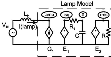
Fig. 3. SPICE-compatible equivalent circuit of a fluorescent lamp.
