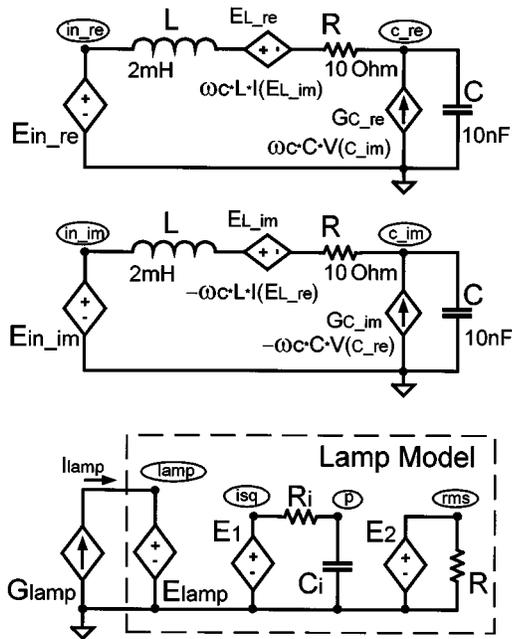
Fig. 12. Envelope simulation SPICE-compatible equivalent circuits of separated ballast-lamp system operating in open loop (Fig. 11).
