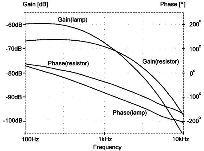
Fig. 7. Simulated small-signal response of the experimental ballast (Fig. 6) loaded by a resistor (150 Ohm) and a fluorescent lamp load.
