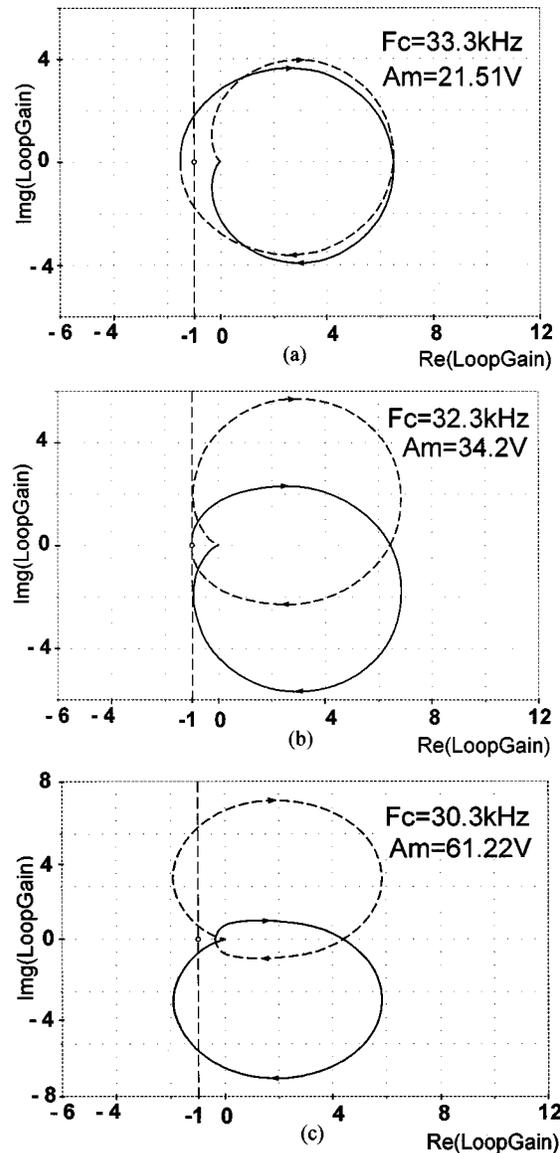
Fig. 13. Nyquist plots of the LoopGain for different values of carrier frequency: (a)  $F_c = 33.3$  kHz (b)  $F_c = 32.3$  kHz. (c)  $F_c = 30.3$  kHz.
