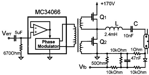
Fig. 6. Experimental ballast-lamp system.
