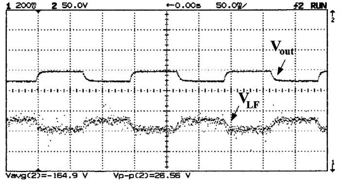
Fig. 14. PLL response under closed loop conditions. Amplitude of  $V_{out}$  is equal to  $A_1$  of Fig. 13.  $V_{LF}$  is the output voltage of the loop filter, (VCO input, Fig. 7).
