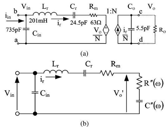
Fig. 2. Equivalent circuits of a PT: (a) original equivalent circuit and (b) simplified equivalent circuit reflecting secondary to the primary side. Values are for PXE43, Philips, operating around 73 kHz.
