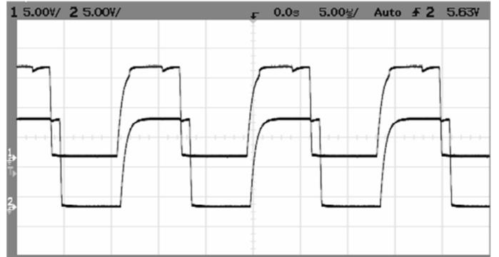
Fig. 10.  $V_3$  (upper trace) and  $V_4$  (lower trace) of the comparators outputs (see Fig. 6).
