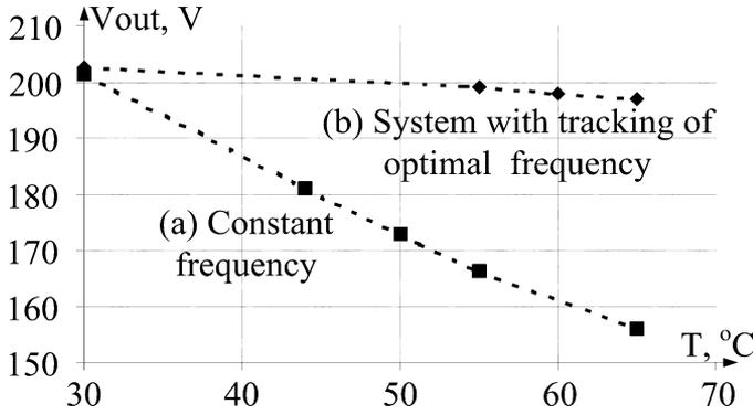
Fig. 11. Output voltage versus PT temperature. (a) Constant frequency operation. (b) With proposed frequency tracking scheme.
