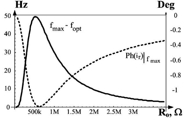
Fig. 4. Phase of  $i_r$  when  $f = f_{\max}$  (dashed-line), and difference between  $f_{\max}$  and  $f_{\text{opt}}$  (solid line).
