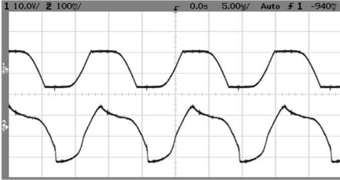
Fig. 8.  $V_{in}$  (upper trace) and  $V_2$  (lower trace) (see Fig. 6) at the series resonant frequency.
