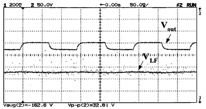
Fig. 15. Open loop response when the drive frequency is  $f_1$ —the frequency of resonance when  $R_L = 1.2$  MΩ. Amplitude of  $V_{out}$  is equal to  $A_2$  of Fig. 13.  $V_{LF}$  is constant voltage to the VCO input (Fig. 7).
