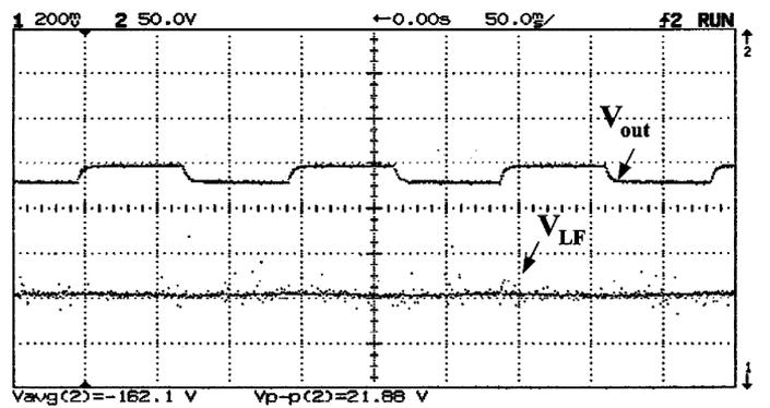
Fig. 16. System without PLL control. Drive frequency is  $f_2$ —the frequency of resonance with  $R_L = 1.76$  MΩ. Amplitude of  $V_{out}$  is equal to  $A_3$  of Fig. 13.  $V_{LF}$  is constant voltage to the VCO input (Fig. 7).
