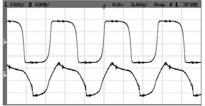
Fig. 9.  $V_1$  (upper trace) and  $V_2$  (lower trace) at the series resonant frequency. (See Fig. 6).
