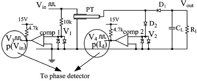
Fig. 6. Proposed method for extracting the phase signals of  $V_{in}$  and  $i_r$ .
