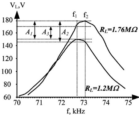
Fig. 13. Steady state output voltage as a function of the operation frequency  $f$ , for two values of the load resistance  $R_L$ . ( $V_{in} = 20.3$  V).
