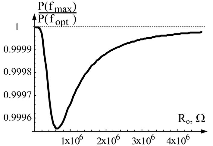
Fig. 5. The ratio between the output power of PT driven at  $f_{\text{opt}}$  to the output power at  $f_{\max}$  as a function of  $R_o$ .
