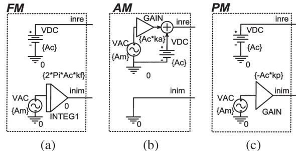
Fig. 6. PSPICE implementation of the decomposed sources for AC-sweep envelope simulation. Real and imaginary components of the source for small-signal envelope simulation for (a) FM, (b) AM, and (c) PM.  $A_c$  is the amplitude of the carrier wave,  $A_m$  is the amplitude of the modulating signal,  $k_f$  is the coefficient of frequency modulation,  $k_a$  is the coefficient of amplitude modulation, and  $k_p$  is the coefficient of phase modulation.
