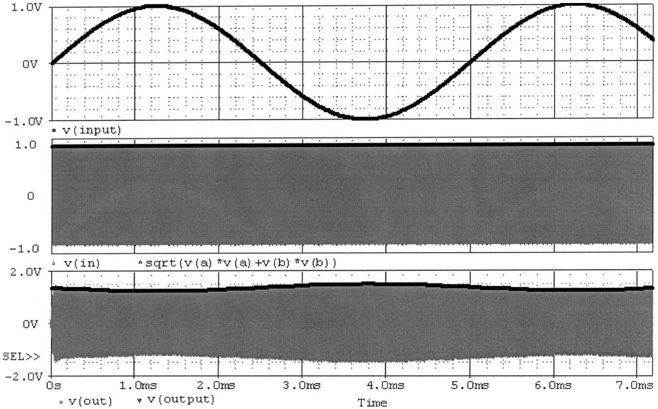
Fig. 5. Transient and envelope-simulation results for FM modulation. Upper curve: modulating signal; middle curves: frequency-modulated input carrier signal (gray) and envelope of the input signal (black line); and lower plot: PT's output signal (gray curve) and its envelope (black curve) obtained by the envelope-simulation model of Fig. 4.
