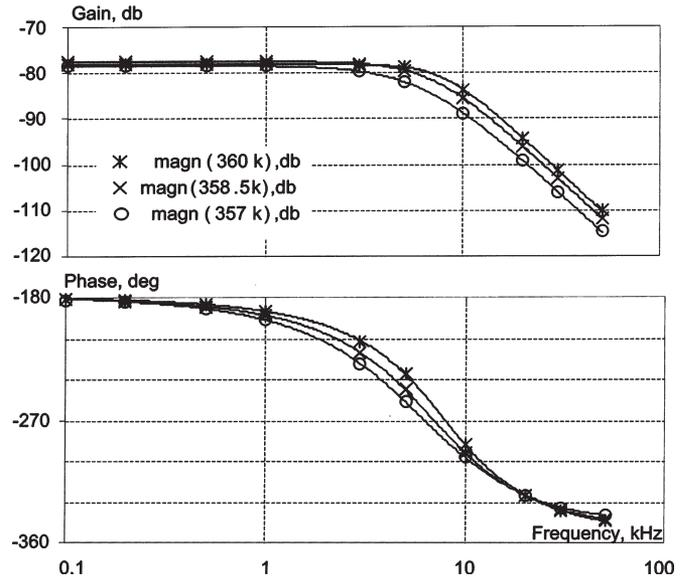
Fig. 8. Small-signal (ac) simulation results of the PT phasor model Fig. 4 excited by an FM signal (lines) compared to the results of multiple runs of transient analysis (symbols) for different carrier frequencies  $f_c$ .
