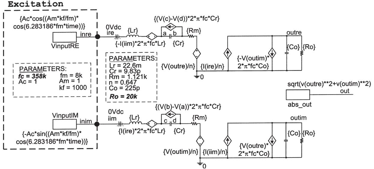
Fig. 4. Schematics of envelope-simulation model of the piezoelectric transformer circuit (Fig. 3) excited by a frequency-modulated signal (PSPICE/OrCAD evaluation Version 9.2).
