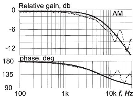
Fig. 10. Small-signal transfer function of the experimental PT under AM excitation. Solid line: small-signal envelope simulation; dashed line: experimental; and carrier frequency: 353 kHz.
