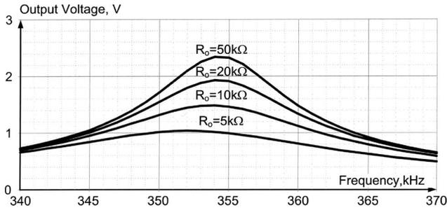
Fig. 7. Steady-state output voltage as a function of excitation (carrier) frequency of the simulation model (Fig. 4) for different loads  $R_o$  obtained by applying dc-envelope analysis.
