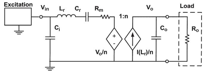
Fig. 3. Equivalent circuit of a piezoelectric transformer loaded by a resistor  $R_o$  and driven by a modulated signal (AM, FM, or PM).
