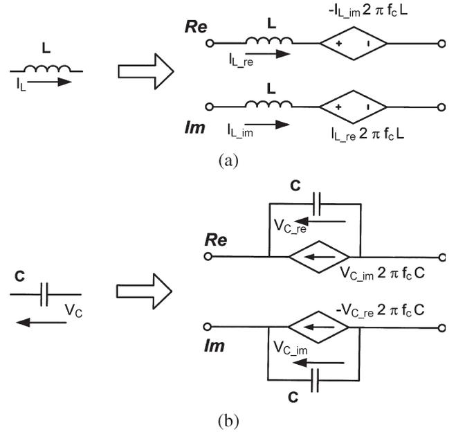
Fig. 2. Replacement of reactive elements by equivalent circuits for envelope simulation. (a) Replacing an inductor by an inductor and dependent voltage source. (b) Replacing a capacitor by a capacitor and dependent current source.
