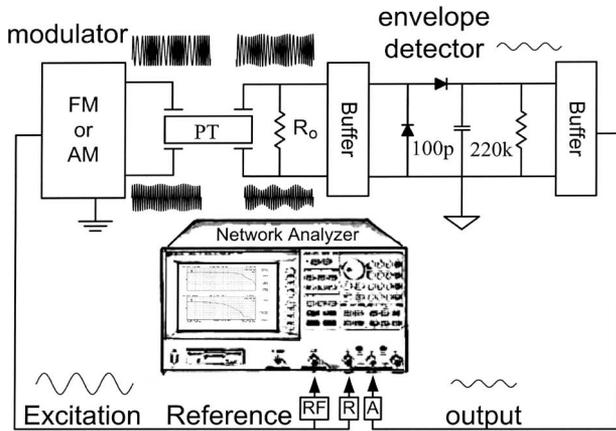
Fig. 9. Experimental setup. The network analyzer measures the ratio between the signals ( $A$ )—envelope of the output signal, and the reference terminal ( $R$ ) which is connected to the excitation port ( $RF$ ).
