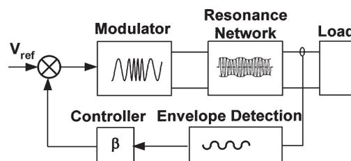
Fig. 1. Resonant converter under closed-loop control.
