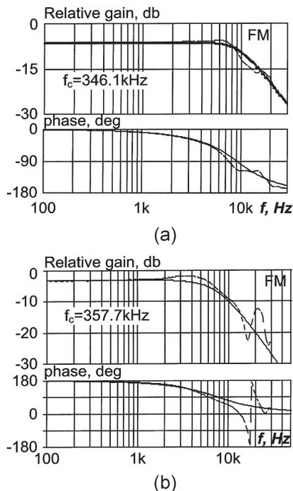
Fig. 11. Small-signal transfer function of the experimental PT under FM excitations. Solid line: small-signal envelope simulation; dashed line: experimental; carrier frequency. (a)  $f_c = 346.1$  kHz. (b)  $f_c = 357.7$  kHz.
