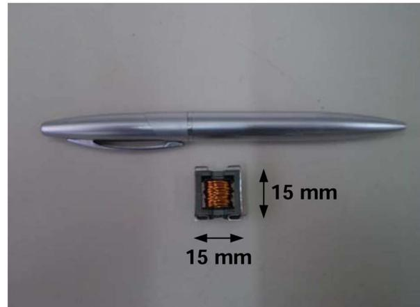
Fig. 15. Realization and the relative dimensions of a 1-mH resonant inductor: EFD 15 core (Philips), 35 turns of AWG #24. Dimensions of inductor: 15 mm  $\times$  15 mm.
