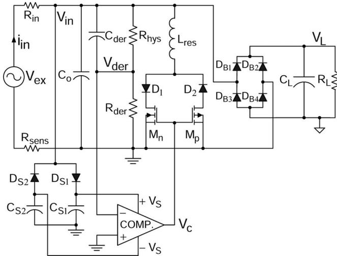
Fig. 6. Circuit diagram of experimental setup with dummy current source.
