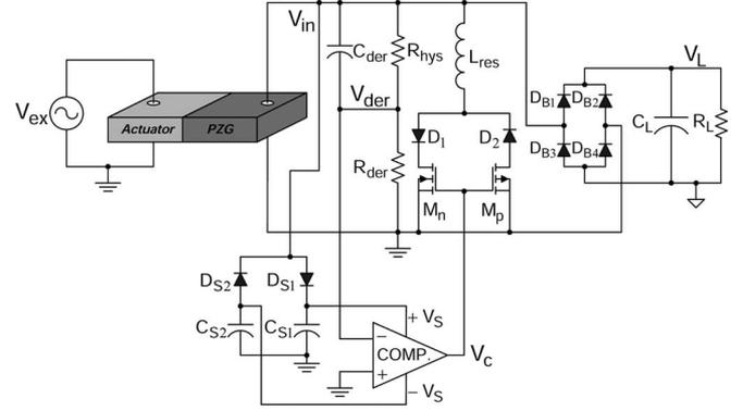
Fig. 10. Circuit diagram of experimental setup with PZG.
