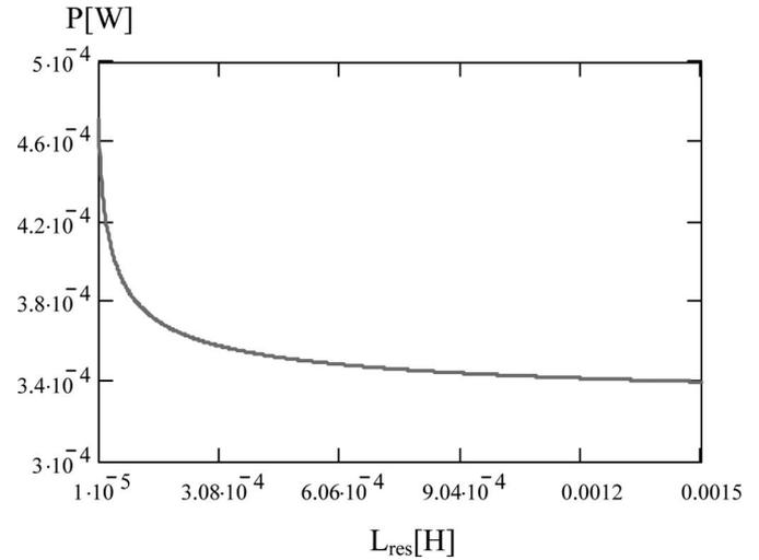
Fig. 14. Power losses calculated as sum  $P_{R_r( loss)} + P_{D( loss)}$  as a function of  $L_{res}$  for:  $f_s = 185$  Hz;  $V_{in(pk)} = 3.5$  V;  $t_D = 0.315$  ms;  $C_o = 330$  nF;  $I_P = 2$  mA;  $V_D = 0.5$  V, and  $R_r = 1 \Omega$ .
