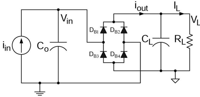
Fig. 2. General topology of a capacitive current source loaded by a conventional diode bridge rectifier circuit.
