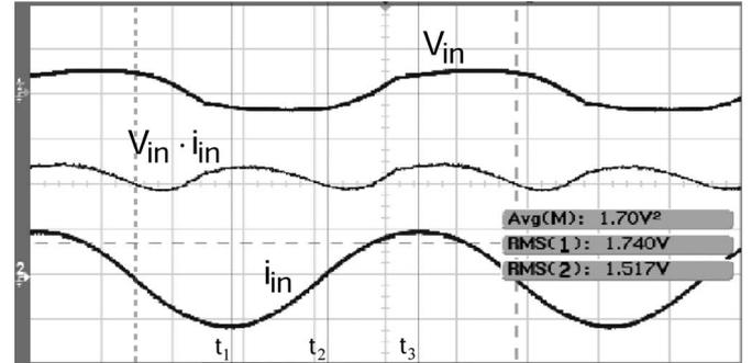
Fig. 7. Experimental waveforms of the standard rectifier. Measured input power: 1.7 mW. Vertical scales:  $V_{in} = 5$  V/div; and  $i_{in} = 2$  mA/div.
