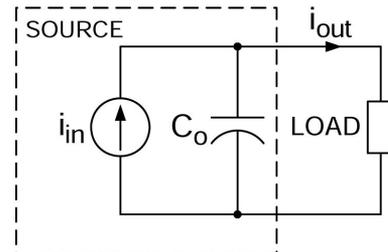
Fig. 1. Electrical equivalent circuit of capacitive current source driving a load.
