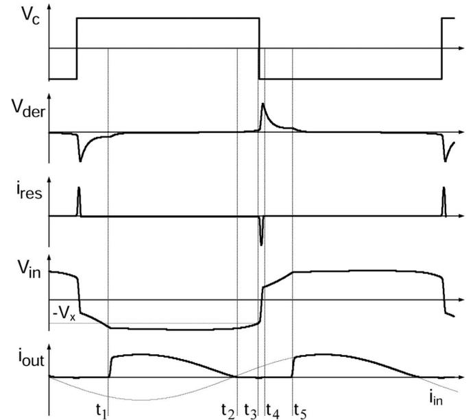
Fig. 5. Key waveforms of the resonant rectifier circuit.
