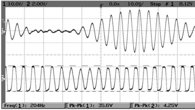
Fig. 11. Experimental waveforms of the PZG under AM excitation connected to the standard rectifier.  $V_{ex}$  (upper trace) and  $V_{in}$  (lower trace) (see Fig. 10).
