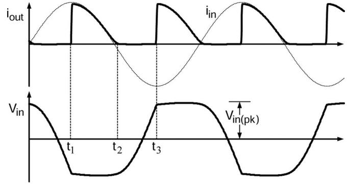
Fig. 3. Typical waveforms of diode bridge rectifier circuit.
