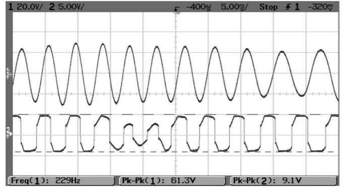
Fig. 13. Experimental waveforms of the PZG under FM excitation connected to the resonant rectifier.  $V_{ex}$  (upper trace) and  $V_{in}$  (lower trace) (see Fig. 10).
