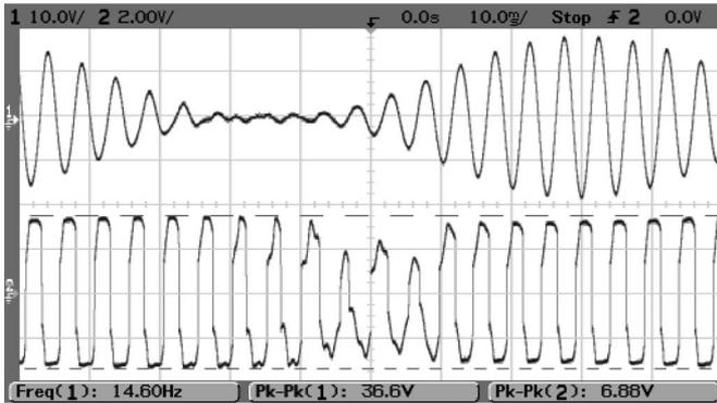
Fig. 12. Experimental waveforms of the PZG under AM excitation connected to the resonant rectifier.  $V_{ex}$  (upper trace) and  $V_{in}$  (lower trace) (see Fig. 10).
