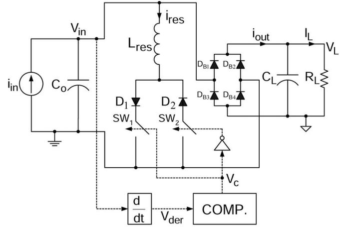
Fig. 4. Proposed resonant rectifier circuit.
