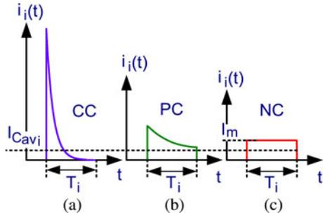
Fig. 4. Possible charging current shapes. (a) Complete charge (CC). (b) Partial charge (PC). (c) No charge (NC).
