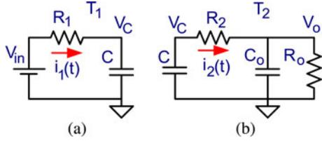
Fig. 2. Subcircuits of the SCC of Fig. 1. (a) Duration  $T_1$ ; (b) Duration  $T_2$ .
