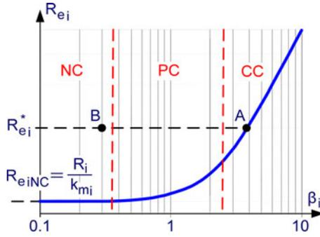
Fig. 6. Behavior of equivalent resistance  $R_{ei}$  of a subcircuit. Smooth curve: (8). “A” point: CC operation. “B” point: NC operation of emulating subcircuit.
