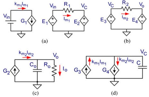
Fig. 5. Average equivalent circuit model of the 1:1 SCC. (a) Emulation of first row of matrix (8). (b) Emulation of second row of (8). (c) Output section. Third row of (8). (d) Capacitor charge balance. Fourth row of (8).
