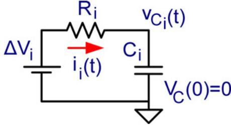
Fig. 3. Generic capacitor-charging equivalent circuit.
