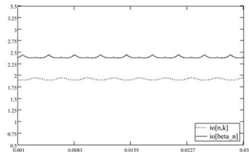
**Fig. 10** MathCAD's steady-state waveforms of the output current  $i_o$  with the following parameters:  $L_o = 1.5 \text{ mH}$ ,  $R_o = 20.3 \Omega$ ,  $f_L = 50 \text{ Hz}$ ,  $f_s = 30 \text{ kHz}$ ,  $V_{LL} = 100 \text{ V}$ ,  $V_o = 12.4 \text{ V}$  and  $M = 0.65$
