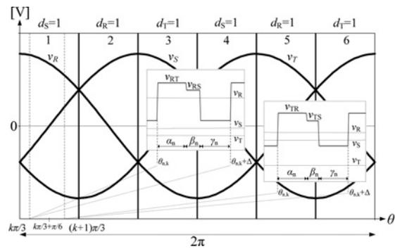
**Fig. 2** Input phase voltages,  $v_R$ ,  $v_S$ ,  $v_T$ , divided into six sectors of  $\pi/3$  and voltage changes during switching interval  $\Delta$
