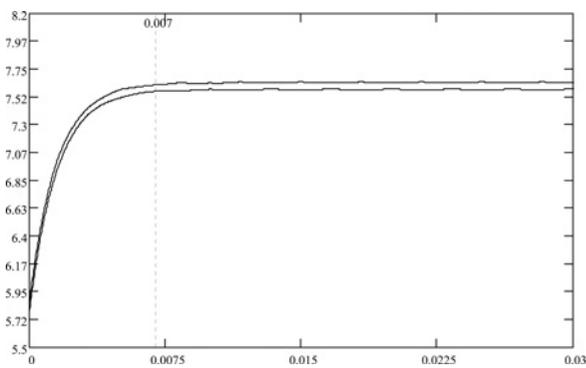
**Fig. 16** MathCAD's waveform of the output current  $i_o$  for a step  $\delta_m = 0.2$  in modulation index,  $M = 0.5-0.7$  with the same parameters as used in Fig. 14
