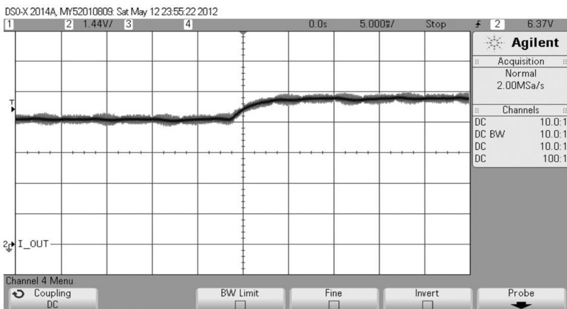
**Fig. 13** Experimental waveform of the output current  $i_o$  for a step  $\delta_m = 0.1$  in modulation index,  $M = 0.5$  to  $M = 0.6$  with the following parameter values:  $L_o = 12$  mH,  $R_o = 8 \Omega$ ,  $V_o = 0$  V,  $f_L = 50$  Hz,  $f_s = 30$  kHz, and  $V_{LL} = 100$  V
