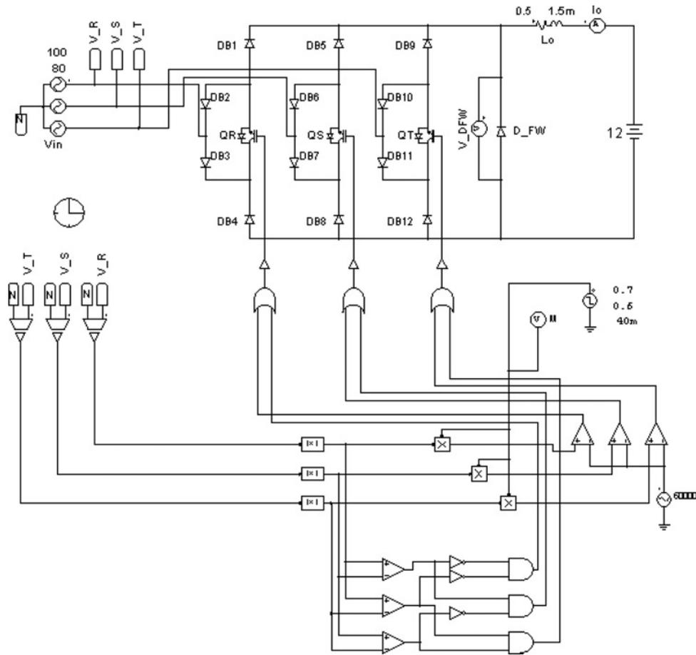
Fig. 5 Simulation circuit of the rectifier and its control elements
