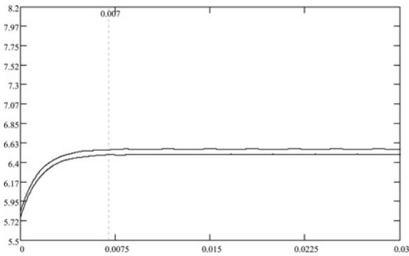
**Fig. 15** MathCAD's waveform of the output current  $i_o$  for a step  $\delta_m = 0.1$  in modulation index,  $M = 0.5-0.6$  with the same parameters as used in Fig. 13
