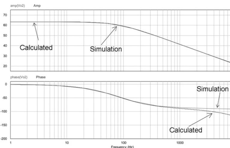
**Fig. 9** Calculated frequency response of the power stage plant  $G(z)$  and simulated frequency response  $G(f)$  obtained from AC analysis in PSIM with the following parameter values
