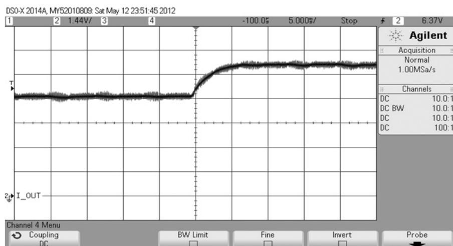
**Fig. 14** Experimental waveform of the output current  $i_o$  for a step  $\delta_m = 0.2$  in modulation index,  $M = 0.5$  to  $M = 0.7$  with the following parameter values:  $L_o = 12$  mH,  $R_o = 8 \Omega$ ,  $V_o = 0$  V,  $f_L = 50$  Hz,  $f_s = 30$  kHz, and  $V_{LL} = 100$  V
