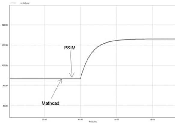
**Fig. 8** Computed and simulated output current response to a step  $\delta_m = 0.1$  in modulation index with the same parameters as used in Fig. 7
