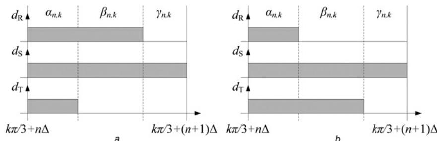
**Fig. 3** Switching pattern and conduction states during one switching period,  $\Delta$ , within
