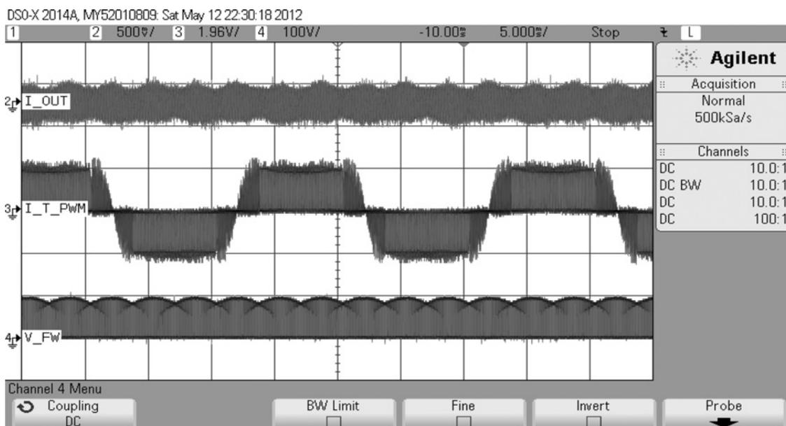
**Fig. 12** Typical experimental waveforms: output current  $i_o$  AC component (upper trace), the current through the switch  $Q_T$  (middle trace), freewheeling diode voltage  $v_{FW}$  (lower trace)
