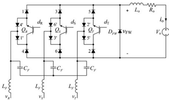
**Fig. 1** General topology of a three-phase buck rectifier
