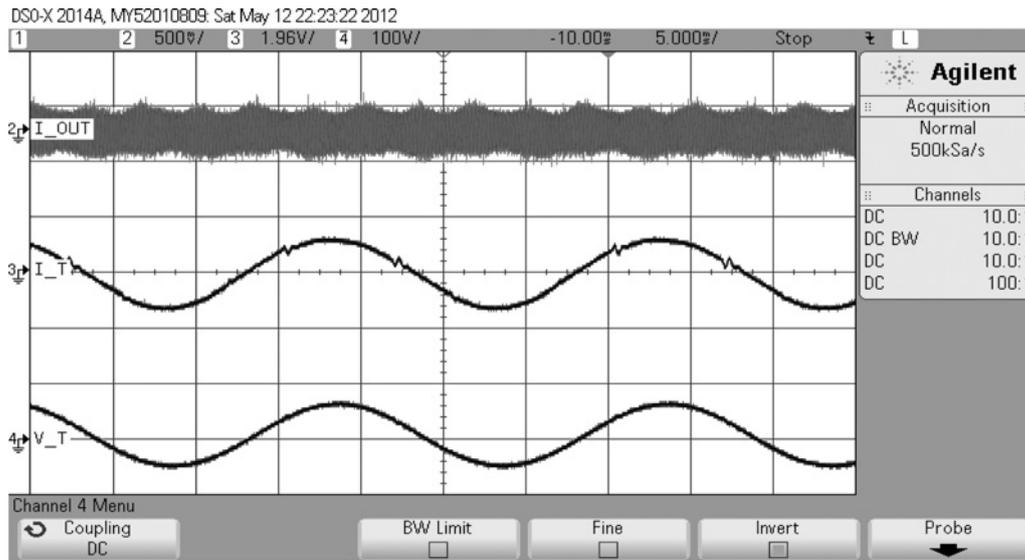
**Fig. 11** Typical experimental waveforms: output current  $i_o$  AC component (upper trace), input phase current  $i_T$  (middle trace) and input phase voltage  $v_T$  (lower trace)
