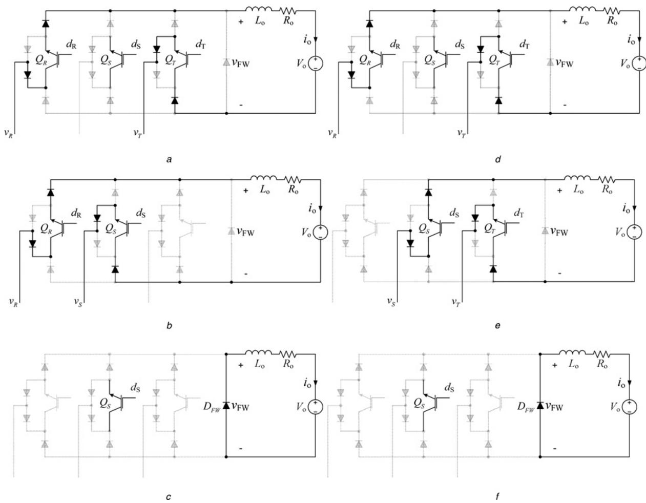
**Fig. 4** Operation topologies of one switching period  $\Delta$
