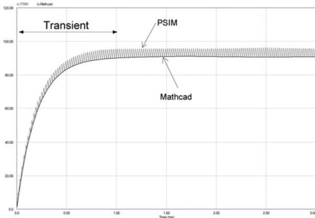
Fig. 6 Computed and simulated output current response of  $i_o[n, k]$  with the following parameter values:  $L_o = 100 \mu\text{H}$ ,  $R_o = 0.5 \Omega$ ,  $f_L = 100 \text{ Hz}$ ,  $f_s = 60 \text{ kHz}$ ,  $V_{LL} = 113 \text{ V}$ ,  $V_o = 12 \text{ V}$  and  $M = 0.6$
