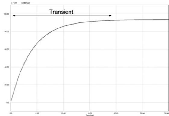
Fig. 7 Computed and simulated output current response of  $i_o[k]$  with the following parameter values:  $L_o = 2 \text{ mH}$ ,  $R_o = 0.5 \Omega$ ,  $f_L = 100 \text{ Hz}$ ,  $f_s = 60 \text{ kHz}$ ,  $V_{LL} = 113 \text{ V}$ ,  $V_o = 12 \text{ V}$  and  $M = 0.6$
