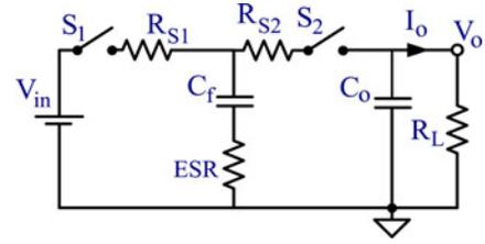
Fig. 5. Simple hard switched 1:1 SCC, switching circuit.
