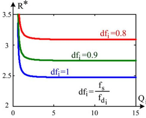
Fig. 18. Dependence of the normalized  $RLC$  subcircuit's equivalent resistance on the subcircuit's quality factor  $Q_i$  with frequency ratio  $df_i$  as a parameter.
