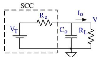
Fig. 1. SCC generic average equivalent circuit.
