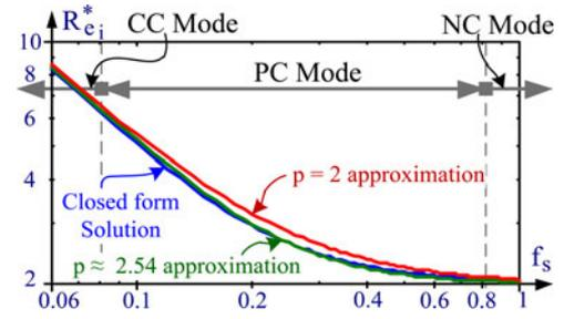
Fig. 16. Comparison of two equivalent resistance empirical equations to closed form solution.
