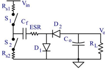
Fig. 11. Inverting 1:1 SCC, switching circuit.
