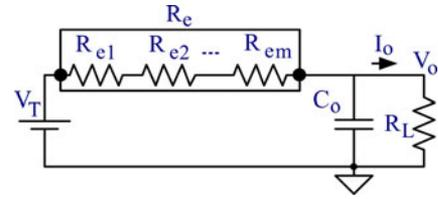
Fig. 3. SCC generic average equivalent circuit that shows the contribution of the partial subcircuits equivalent resistances  $R_{e_i}$  to the total equivalent circuit  $R_e$ . (For the unity SCC example [see Fig. 2(a)],  $R_{e_1}$  is the loss contribution of charge subcircuit and  $R_{e_2}$  is the loss contribution of discharge subcircuit.)
