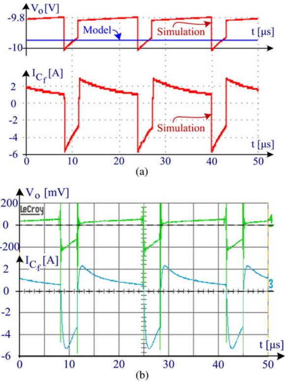
Fig. 21. Hard switched inverting 1:1 SCC waveforms: (a) Full circuit (cycle by cycle) simulation and model calculation. (b) Experimental details.
