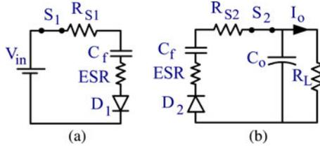
Fig. 12. Hard switched inverting 1:1 SCC operational phases: (a) Charge. (b) Discharge.
