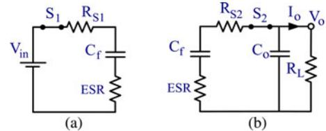
Fig. 6. Hard switched 1:1 SCC operation phases: (a) Charge. (b) Discharge.
