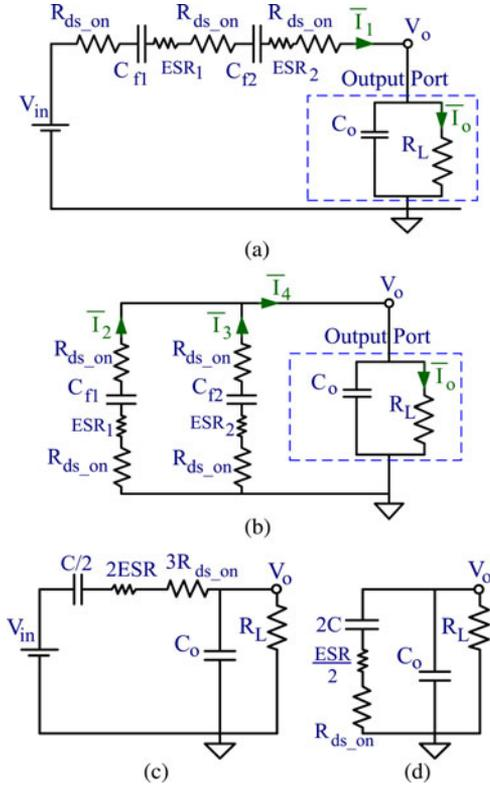
Fig. 10. Step down 3:1 SCC operation phases: (a) Phase 1. (b) Phase 2. (c) Simplified subcircuit of phase 1. (d) Order reduction of the subcircuit of phase 2. Arrows: average subcircuits currents.
