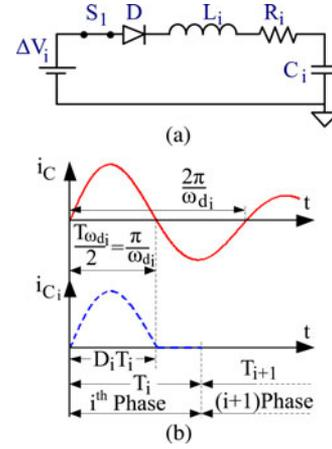
Fig. 4. Resonant charge/discharge process: (a) Basic and generic, instantaneous  $RLC$  circuit. (b) Current waveforms: straight (red) trace—resonant current waveform with no diode. Dashed (blue) trace—actual capacitor charging current waveform with blocking diode.
