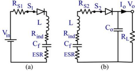
Fig. 8. Soft switched 1:1 SCC operation phases: (a) Charge. (b) Discharge.
