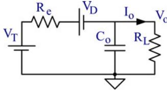
Fig. 13. SCC generic average equivalent circuit including diode losses.
