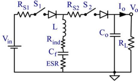
Fig. 7. Simple soft switched 1:1 SCC, switching circuit.
