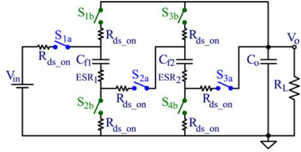
Fig. 9. Step down 3:1 SCC, switching circuit.
