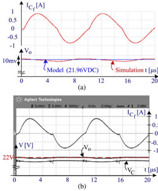
Fig. 20. Soft switched 1:1 unity converter waveforms: (a) Simulation and model. (b) Experimental details.
