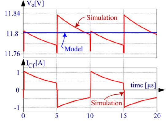
Fig. 19. Simulated and model calculated results of hard switched 3:1 step-down SCC: Upper traces—output voltage. Lower trace—capacitor current  $C_{f1}$ .
