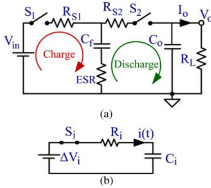
Fig. 2. Unity SCC and the basic charge/discharge RC subcircuit: (a) Unity SCC—switching circuit, (b) Basic and generic, instantaneous RC subcircuit.
