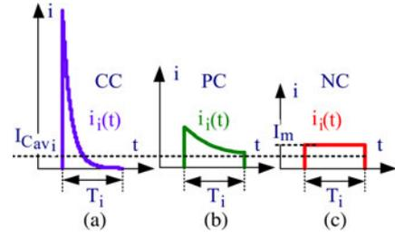
Fig. 14. Charge/discharge instantaneous current waveforms: (a) Complete charge—"CC" mode. (b) Partial charge—"PC" mode. (c) No charge—"NC" mode.
