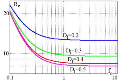
Fig. 17. Dependence of the equivalent resistance on the duty cycle  $D$  as a function of normalized frequency in a two phase hard switched unity SCC.
