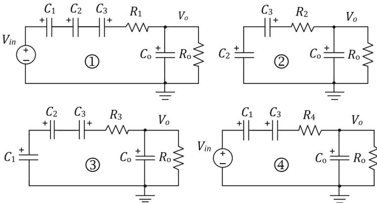
**Fig. 2** Topologies of the SCC with the conversion ratio  $M = 3/8$
